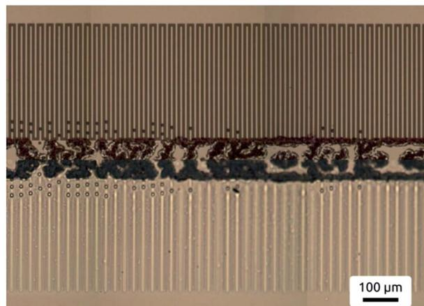
Fig. 3 Microscopy image demonstrating the ease of pattern replication over larger areas. The bottom panel shows the PVME film, the top panel the electrode pattern. After pattern formation the two plates have been separated and the top electrode has been folded upwards. The features dividing top and bottom panel are the electrode spacers. The mirror plane character of the horizontal line is visible.
