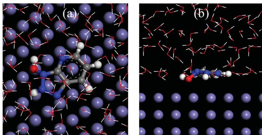
Fig. 13 Equilibrium adsorption configuration for HOATH<sup>+</sup> on the Fe (110) surface: (a) top and (b) side views.
