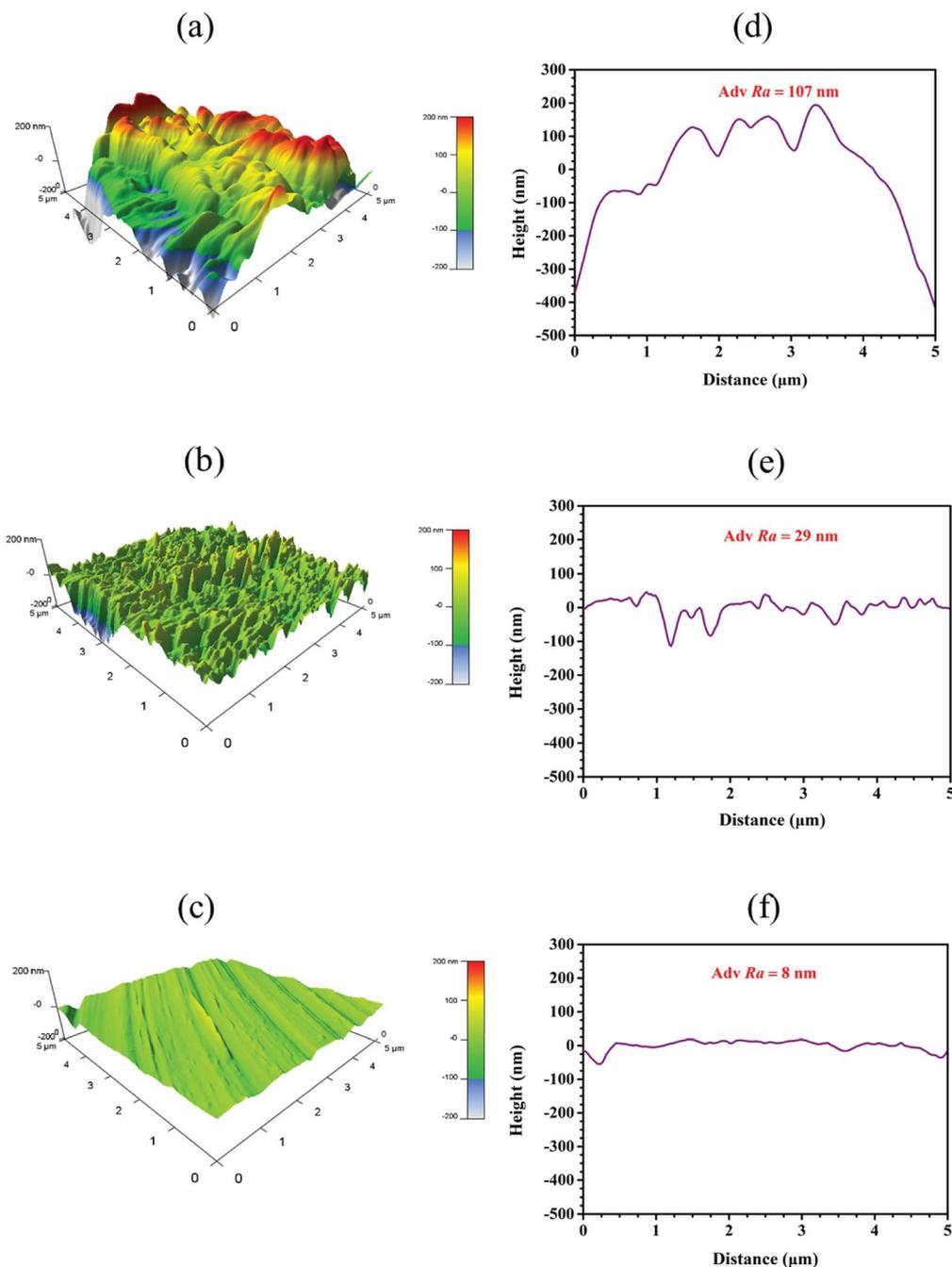
Fig. 10 The images of AFM 3D and height profile plots of corroded steel (a and d) without HOAT, steel (b and e) with 10 mM HOAT in 1 M  $\text{H}_2\text{SO}_4$  solution and new polished steel (c and f) for 2 h at 298 K.
