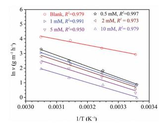
Fig. 7 The plots of Arrhenius for steel in 1 M H<sub>2</sub>SO<sub>4</sub> without and with diverse concentrations of HOAT.
