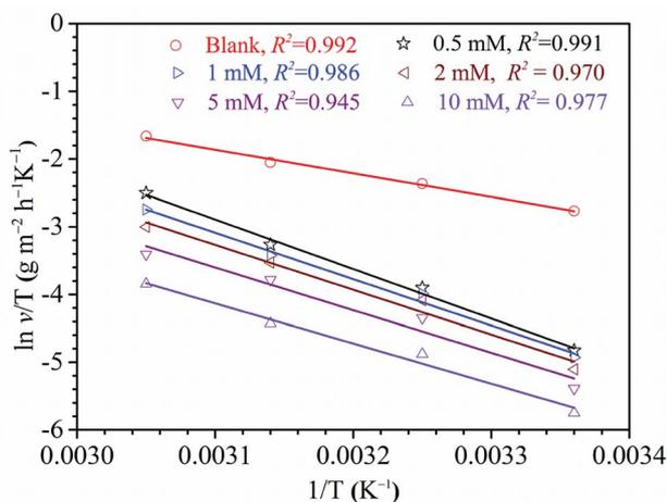
Fig. 8 The plots of transition state to steel in 1 M H<sub>2</sub>SO<sub>4</sub> without and with diverse concentrations of HOAT.
