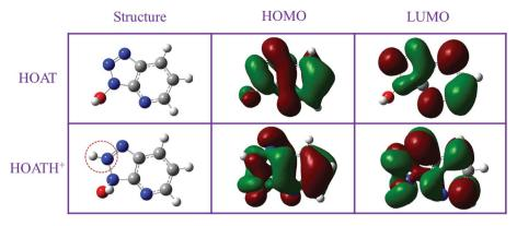
Fig. 11 The optimized structures, HOMO and LUMO of the HOAT and HOATH<sup>+</sup>.
