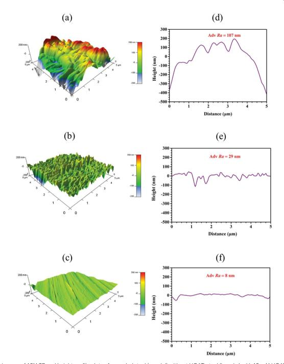
Fig. 10 The images of AFM 3D and height profile plots of corroded steel (a and d) without HOAT, steel (b and e) with 10 mM HOAT in 1 M  $_2$ SO<sub>4</sub> solution and new polished steel (c and f) for 2 h at 298 K.
