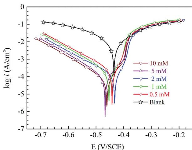
**Fig. 2** Tafel curves for mild steel at 298 K in 1 M H<sub>2</sub>SO<sub>4</sub> without and with different concentrations of HOAT.
