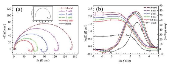
Fig. 3 EIS plots of the mild steel at 298 K in 1 M H<sub>2</sub>SO<sub>4</sub> solution without and with diverse concentrations of HOAT: (a) Nyquist and (b) Bode plots.
