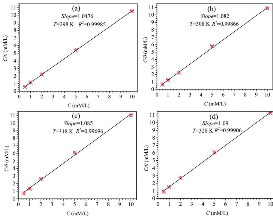
Fig. 5 The plots of Langmuir isotherm for mild steel in 1 M H<sub>2</sub>SO<sub>4</sub> including different concentrations of HOAT at diverse temperatures (298 K, 308 K, 318 K and 328 K).
