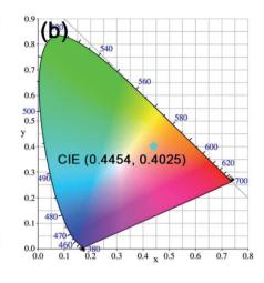
Fig. 9 (a) EL spectrum of the fabricated white LED device with 395 nm near-UV chip, BAM:Eu<sup>2+</sup> blue phosphors, (Ba,Sr)<sub>2</sub>SiO<sub>4</sub>:Eu<sup>2+</sup> green phosphors, and BYO:0.25Eu<sup>3+</sup> red phosphors under 60 mA current. Inset shows the fabricated LED device and corresponding luminescent image. (b) CIE chromaticity diagram of the fabricated white LED device.
