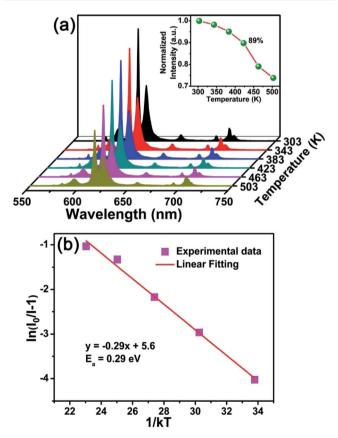
Fig. 8 (a) Temperature-dependent PL spectra of BYO:0.25Eu $^{3+}$  phosphors excited at 396 nm. Inset shows the normalized PL intensity of BYO:0.25Eu $^{3+}$  phosphors as a function of temperature. (b) Plot of ln  $[(I_0/I)-1]$  vs. 1/kT.
