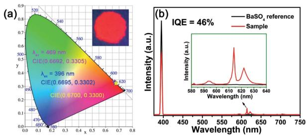
Fig. 7 (a) CIE chromaticity diagram of BYO:0.25Eu $^{3+}$  phosphors under 396 and 469 nm excitation. Inset shows the photograph of BYO:0.25Eu $^{3+}$  under a 365 nm UV lamp. (b) Excitation line of BaSO<sub>4</sub> and the emission spectrum of BYO:0.25Eu $^{3+}$  phosphors collected using an integrating sphere. Inset shows a magnification of the emission spectrum in the 580–640 nm range.
