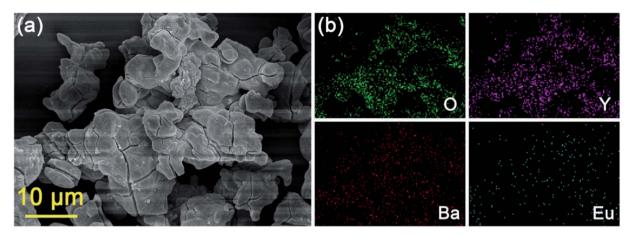
Fig. 3 (a) FE-SEM image of BYO:0.25Eu<sup>3+</sup> phosphors. (b) Elemental mapping of BYO:0.25Eu<sup>3+</sup> phosphors.
