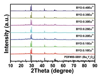
Fig. 1 XRD patterns of BYO: $xEu^{3+}$  (x = 0.10, 0.15, 0.20, 0.25, 0.30,0.35, and 0.40) phosphors. The standard data of Ba<sub>3</sub>Y<sub>4</sub>O<sub>9</sub> (PDF#89-5891) was shown as reference.
