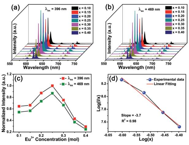
Fig. 5 (a) PL spectra of BYO:xEu<sup>3+</sup> phosphors under 396 nm excitation. (b) PL spectra of BYO:xEu<sup>3+</sup> phosphors under 469 nm excitation. (c) Normalized PL intensity of BYO:xEu<sup>3+</sup> phosphors as a function of Eu<sup>3+</sup> concentration. (d) Plot of log(I/x) vs. log(x) of Eu<sup>3+</sup> ions in BYO:xEu<sup>3+</sup> phosphors excited at 396 nm and monitored at 614 nm.
