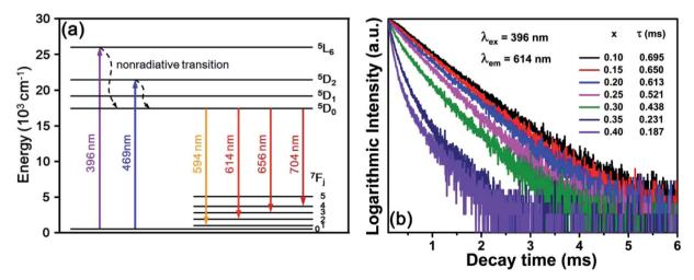
Fig. 6 (a) Energy level diagram of Eu<sup>3+</sup> ions. (b) Decay curves of BYO:xEu<sup>3+</sup> phosphors excited at 396 nm and monitored at 614 nm.
