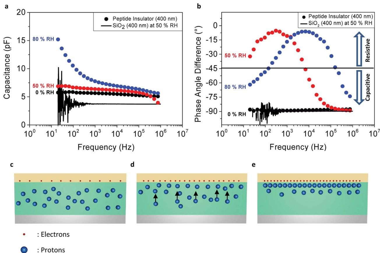
Fig. 3 Measurement of capacitance and phase angle of the peptide insulator. (a) Capacitance plots and (b) phase angle plots of the peptide insulator and the reference  $\text{SiO}_2$  as a function of AC frequency and RH conditions. Schematics of the behavior of protons in the peptide insulator under (c) high-frequency, (d) mid-frequency, and (e) low-frequency AC perturbation.
