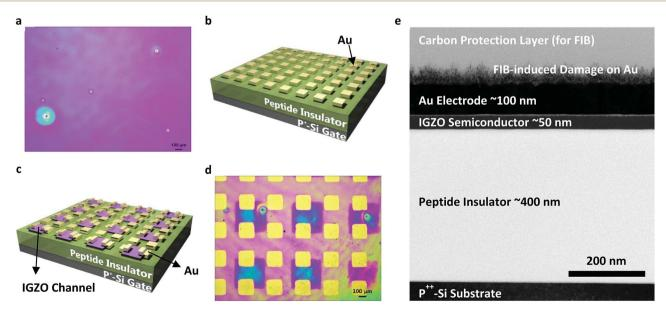
Fig. 2 (a) Optical microscopic image of the RH-controlled peptide film. 3-D structure of (b) MIM sample and (c) TFT sample. (d) Top-view optical microscopic image and (e) side-view TEM image of IGZO TFTs with the peptide insulator.
