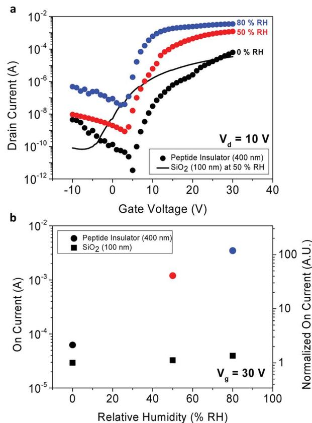
Fig. 6 Electrical characteristics of TFT samples. (a) Comparison of the transfer curves and (b) on-current level of the peptide TFT samples with the reference  $\text{SiO}_2$  samples in various humidity conditions.
