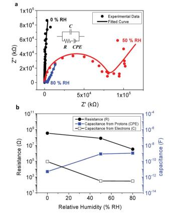
Fig. 4 Comparison of the experimental results and simulated results. (a) Complex impedance plots of the experimental results (dots), fitted curves (line), and according equivalent circuit (inset). (b) Comparison of changes in each circuit element used in the equivalent circuit as RH condition changed.
