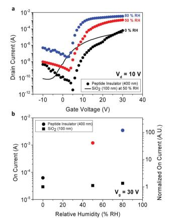
Fig. 6 Electrical characteristics of TFT samples. (a) Comparison of the transfer curves and (b) on-current level of the peptide TFT samples with the reference SiO<sub>2</sub> samples in various humidity conditions.
