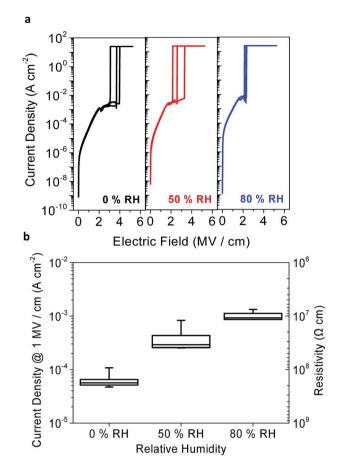
Fig. 5 Dielectric strength and resistivity of the peptide insulator. (a) Breakdown curves and (b) current density graph of the peptide insulator under various RH conditions.
