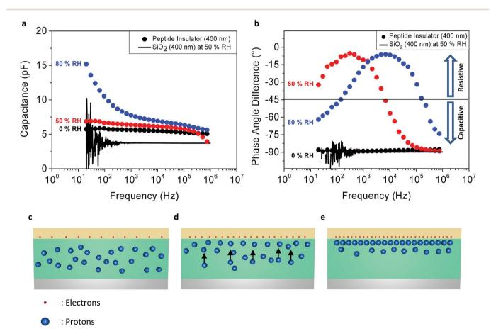
Fig. 3 Measurement of capacitance and phase angle of the peptide insulator. (a) Capacitance plots and (b) phase angle plots of the peptide insulator and the reference SiO<sub>2</sub> as a function of AC frequency and RH conditions. Schematics of the behavior of protons in the peptide insulator under (c) high-frequency, (d) mid-frequency, and (e) low-frequency AC perturbation.
