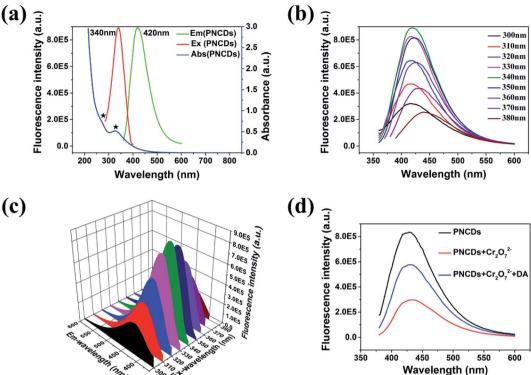
Fig. 3 (a) UV-vis absorption (blue line), PL excitation (red line), and emission (green line) spectra of PNCDs in aqueous solution (0.30 mg mL<sup>-1</sup>). (b) Excitation-dependent PL behavior of PNCDs. (c) 3D wall spectra of the PNCDs with different excitation wavelength. (d) Fluorescence emission spectra of PNCDs at different conditions: PNCDs (black line), PNCDs +  $Cr_2O_7^{2-}$  (red line), PNCDs +  $Cr_2O_7^{2-}$  + DA (blue line)
