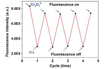
Fig. 6 Fluorescence intensity changes at 340 nm of PNCDs upon alternate addition of concentrations of 160  $\mu$ M Cr(vi) and 160  $\mu$ M DA in PBS (pH: 7.4).
