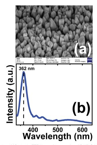
Fig. 1 (a) Depicts the FESEM image of the top surface of GaN/N:GaN/N:HfO $_2$ /SiO $_2$ /p-Si heterostructure nanorods network epitaxially grown on nitridated HfO $_2$  buffer layer, and (b) Photoluminescence (PL) spectra of GaN nanorods network at 325 nm excitation.
