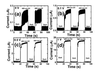
Fig. 3 Show I-t plots for photo-detector device in dark vs. UV laser illumination. (a) and (b) are current response of the photo-detector device at the applied voltage of 0 V & 0.1 V, (c) and (d) at 0.5 V & 1 V.
