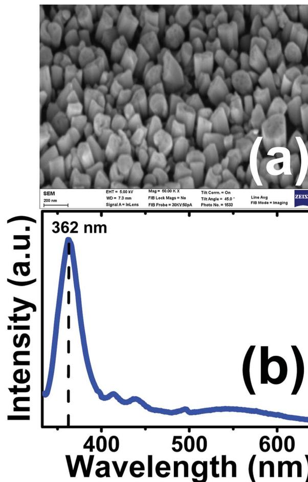
Fig. 1 (a) Depicts the FESEM image of the top surface of GaN/N:Ga/N:HfO<sub>2</sub>/SiO<sub>2</sub>/p-Si heterostructure nanorods network epitaxially grown on nitridated HfO<sub>2</sub> buffer layer, and (b) Photoluminescence (PL) spectra of GaN nanorods network at 325 nm excitation.
