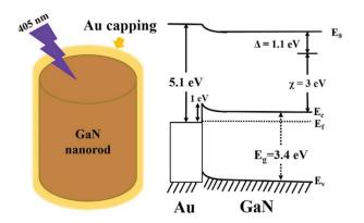
Fig. 4 Depicts the energy band situation for the Au/GaN nanorods interface where the near-UV laser incidents. The left side image shows the nanorods' capping with the semi-transparent Au electrode.
