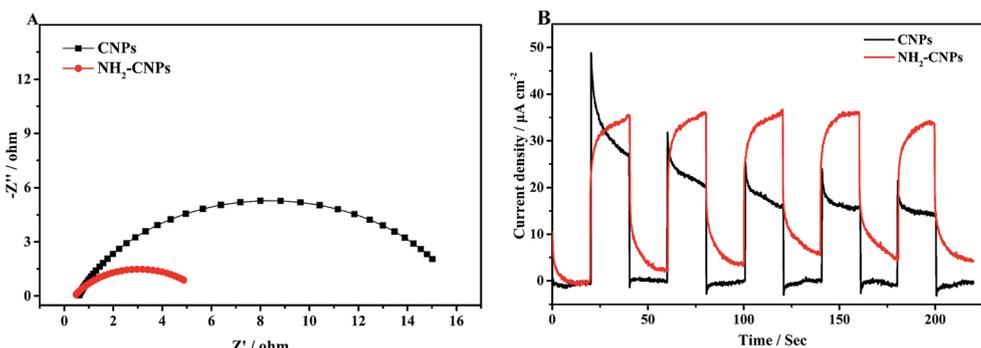
Fig. 7 (A) Nyquist plots of the CNPs (a) and  $\text{NH}_2$ -CNPs (b). (B) The transient photocurrent responses of the CNPs (a) and  $\text{NH}_2$ -CNPs (b) in 0.5 M  $\text{Na}_2\text{SO}_4$  aqueous solution under visible-light ( $\lambda > 420$  nm) irradiation.
