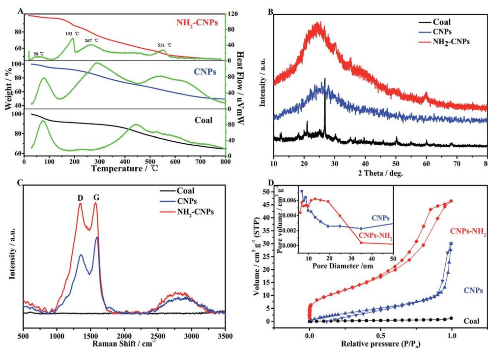
Fig. 3 Physical characterizations of coal powder, CNPs, and NH<sub>2</sub>-CNPs. (A) TG-DTG; (B) XRD; (C) Raman; (D) BET.
