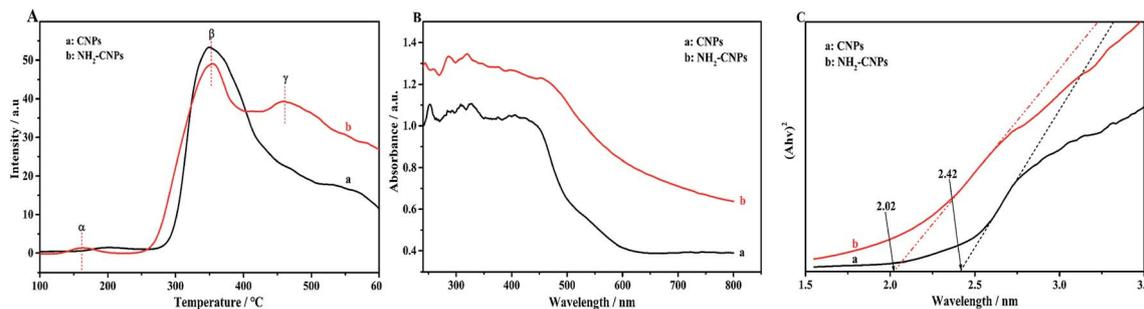
Fig. 6 (A) The CO<sub>2</sub>-TPD profiles of the CNPs (a) and NH<sub>2</sub>-CNPs (b). (B) DR UV-vis spectra of the CNPs (a) and NH<sub>2</sub>-CNPs (b). (C) The calculation of the band gap of the CNPs (a) and NH<sub>2</sub>-CNPs (b) based on the  $(Ah\nu)^2$  versus  $h\nu$  curve.
