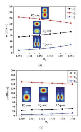
Fig. 6 Light field distribution and the attenuation of  $E_{11}^{x}$  mode,  $E_{12}^{x}$  mode and  $E_{21}^{x}$  mode with different polymer cladding  $n_3$  (h=5 µm) at (a) T=293.15 K and (b) T=303.15 K.
