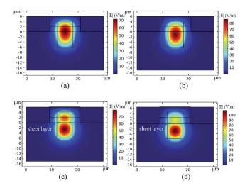
Fig. 3 Optical field distribution of  $E_{11}^{x}$ -polarized light without and with a sheet layer embedded in waveguide core for T = (a and c) 293.15 and (b and d) 303.15 K (structure 1), respectively (electrode heating power (P) = 48.39 mW).
