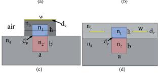
Fig. 1 Three-dimensional structures and two-dimensional cross-sectional structures of polymer-graphene-silica hybrid waveguide with structure (a and c) 1 and (b and d) 2, respectively.
