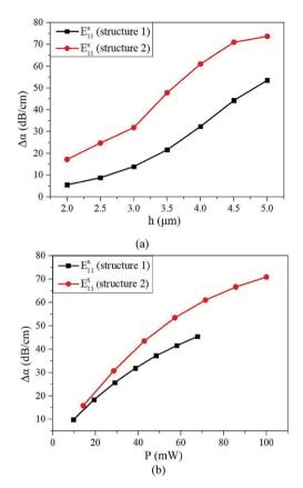
Fig. 5 Curves of the polymer layer height and attenuation variation  $(\Delta \alpha)$  for structure 1 and structure 2 as a function of (a) polymer waveguide height h and (b) electrode heating power P, respectively  $(n_3 = 1.460)$ .
