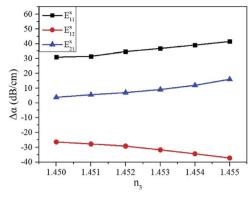
Fig. 7 Relationships between cladding refractive index ( $n_3$ ) and attenuation variation ( $\Delta\alpha$ ) of  $E_{11}^x$ ,  $E_{12}^x$ , and  $E_{21}^x$  modes ( $h=5~\mu m$ ; P=43.86~mW; structure 1).
