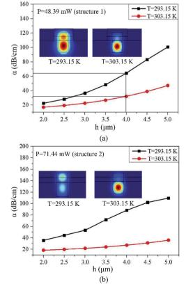
Fig. 4 Light field distribution and attenuation of  $E_{11}^{x}$  mode with different height of polymer layer and electrode temperature ( $n_3 = 1.460$ ) for (a) structure 1 and (b) structure 2, respectively.
