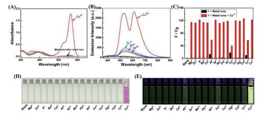
Fig. 1 Spectroscopic changes of 1 (20  $\mu$ M) with the addition of various metal ions in CH<sub>3</sub>CN-H<sub>2</sub>O (9/1, v/v) solution. (A) Absorption spectral changes. (B) Fluorescence emission intensity changes. (C) The fluorescence intensity changes at 610 nm (black bars: 1 with other ions, red bars: 1 with  $Cu^{2+}$  and other metal ions). (D) The color image with the addition of various metal ions. (E) The fluorescence image with the addition of various metal ions
