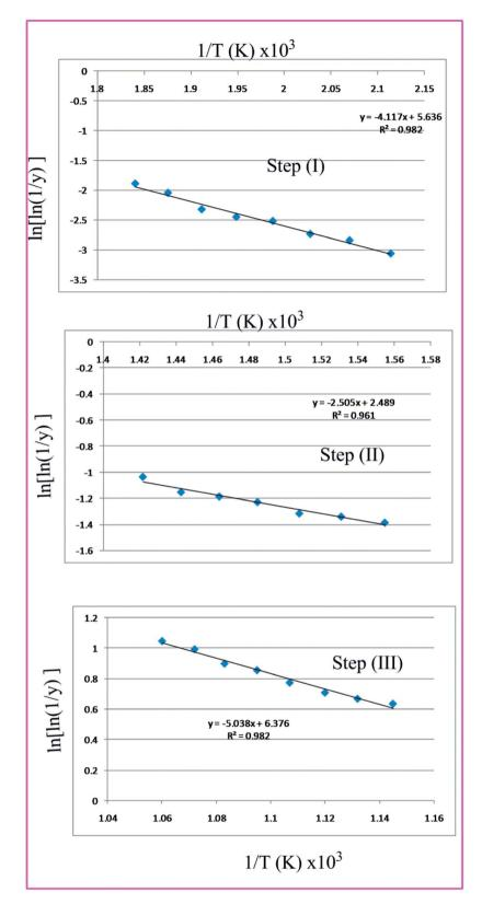
Fig. 11 Broido the three thermal decomposition steps of complex 3.
