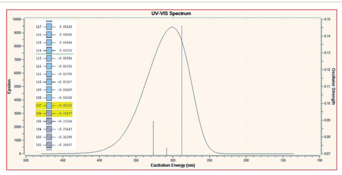
Fig. 5 TD-DFT UV-visible spectrum of ligand II with the overlayed MO levels.
