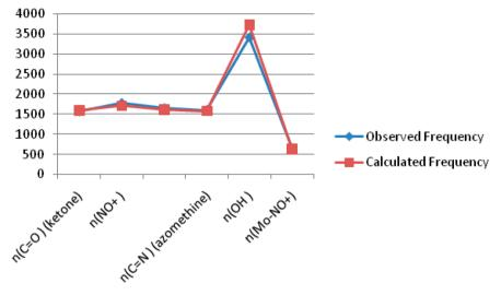
A plot of observed FT-IR frequency versus theoretical data of complex 2.
