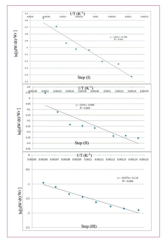
Fig. 8 Freeman Carroll plots for the three thermal decomposition steps of complex 3.
