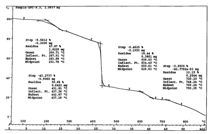
Fig. 7 Thermo-analytical curve of complex 3
