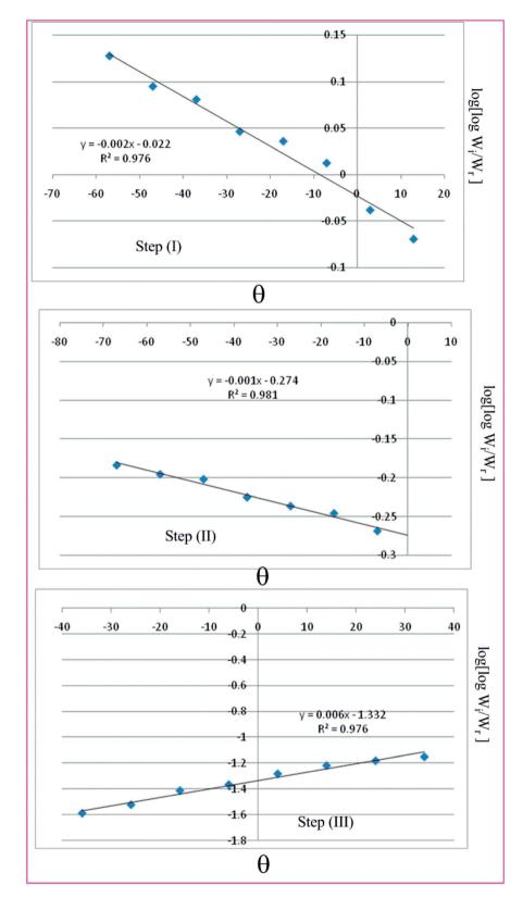
Fig. 9 Horowitz-Metzger plots for the three thermal decomposition steps of complex 3.
