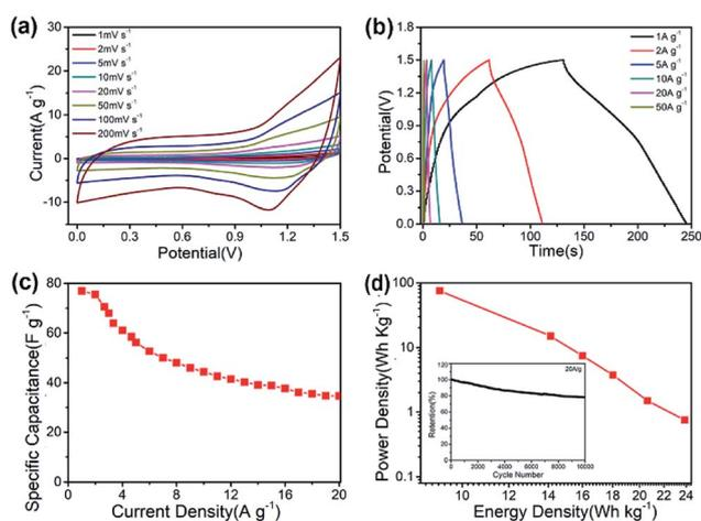
Fig. 7 Electrochemical characterization of a CNF@NiMo-2//AC asymmetric supercapacitor device: (a) CV curves collected at different scan rates ranging from 1 to  $200 \text{ mV s}^{-1}$ ; (b) galvanostatic charge/discharge voltage profiles at different current densities in the voltage range of 0–1.5 V; (c) rate capability; (d) the power density of CNF@NiMo-2//AC ASC device at different energy density; The inset in (d) shows cycling stability at a current density of  $20 \text{ A g}^{-1}$ .
