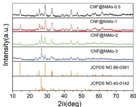
Fig. 1 XRD pattern of different CNF@NiMo samples.
