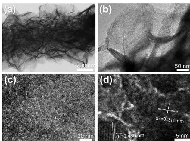
Fig. 3 (a–c) TEM images of CNF@NiMo-2 at different magnification. (d) Corresponding HRTEM image of NiMoO<sub>4</sub> nanosheets on CNFs.
