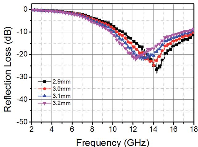
Fig. 6 RL curves of RGO<sub>160</sub>/wax composites, where the filler loading ratio is 5 wt% and the thicknesses are from 2.9 to 3.2 mm.
