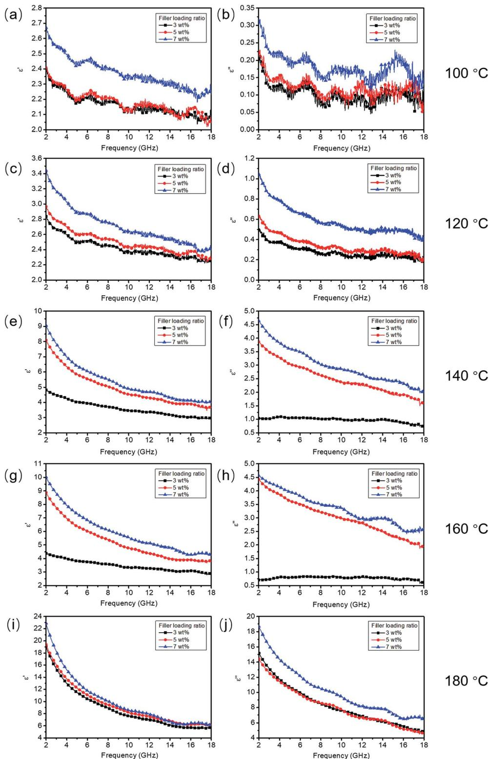
Fig. 3 Frequency-dependent real and imaginary permittivity of RGO<sub>100</sub> (a and b), RGO<sub>120</sub> (c and d), RGO<sub>140</sub> (e and f), RGO<sub>160</sub> (g and h), and RGO<sub>180</sub> (i and j), with filler loading ratios of 3, 5 and 7 wt% in the wax composites.
