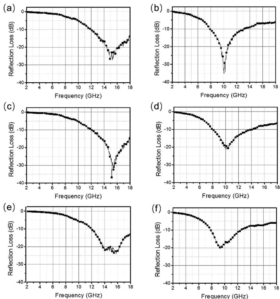
Fig. 8 The thinnest thicknesses to absorb Ku and X bands effectively: RL curves of a composite loaded with 5 wt% RGO<sub>140</sub> (a and b) and RGO<sub>160</sub> (c and d); RL curves of a composite loaded with 7 wt% RGO<sub>160</sub>.
