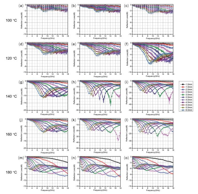
Fig. 4 RL curves of RGO<sub>100</sub> (a–c), RGO<sub>120</sub> (d–f), RGO<sub>140</sub> (g–i), RGO<sub>160</sub> (j–l) and RGO<sub>180</sub> (m–o) with filler loading ratios of 3, 5 and 7 wt% in wax composites.
