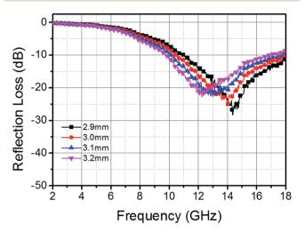
Fig. 6 RL curves of  $RGO_{160}$ /wax composites, where the filler loading ratio is 5 wt% and the thicknesses are from 2.9 to 3.2 mm.
