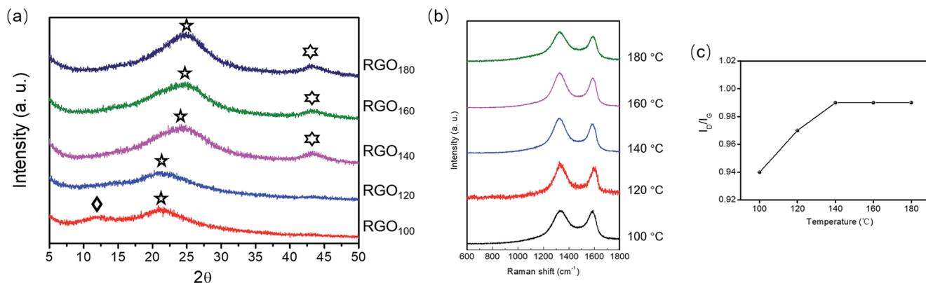
Fig. 1 XRD (a), Raman (b) and  $I_D/I_G$  (c) spectra of RGO<sub>100</sub>, RGO<sub>120</sub>, RGO<sub>140</sub>, RGO<sub>160</sub> and RGO<sub>180</sub>.
