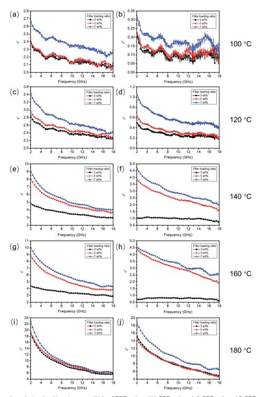
Fig. 3 Frequency-dependent real and imaginary permittivity of RGO $_{100}$  (a and b), RGO $_{120}$  (c and d), RGO $_{140}$  (e and f), RGO $_{160}$  (g and h), and RGO $_{180}$  (i and j), with filler loading ratios of 3, 5 and 7 wt% in the wax composites.
