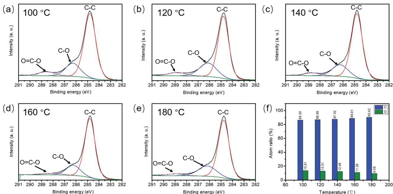
Fig. 2 C 1s spectra of RGO<sub>100</sub> (a), RGO<sub>120</sub> (b), RGO<sub>140</sub> (c), RGO<sub>160</sub> (d) and RGO<sub>180</sub> (e) using XPS, and the ratios of C/O in each sample (f).
