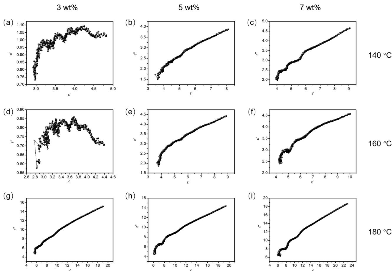
Fig. 7 Cole–Cole plots for the RGO<sub>140</sub>/wax (a–c), RGO<sub>160</sub>/wax (d–f), and RGO<sub>180</sub>/wax (g–i) composites.
