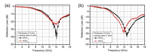
Fig. 5 A comparison of the effective EA bandwidths of composites loaded with 5 wt% and 7 wt% RGO<sub>140</sub> and RGO<sub>160</sub> at the same thickness of 3 mm.
