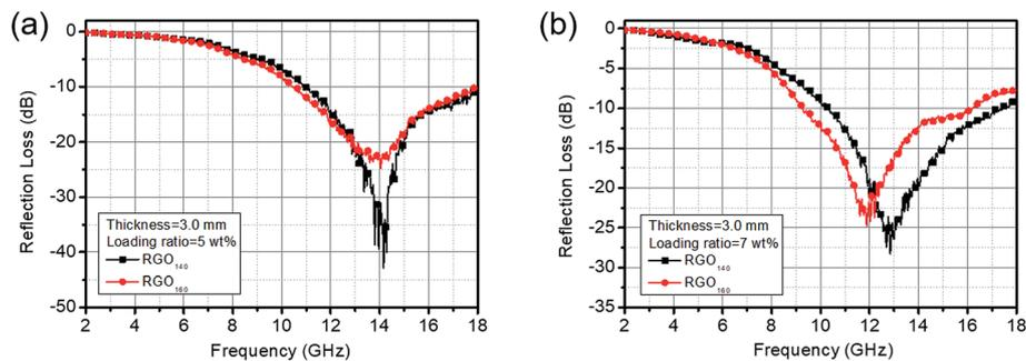
Fig. 5 A comparison of the effective EA bandwidths of composites loaded with 5 wt% and 7 wt% RGO<sub>140</sub> and RGO<sub>160</sub> at the same thickness of 3 mm.
