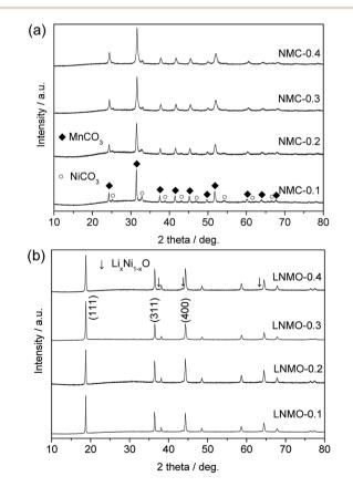
Fig. 1 XRD patterns of carbonate precursors (a) and  $LiNi_{0.5}Mn_{1.5}O_4$  samples (b) synthesized at different reactant concentrations.
