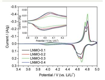
Fig. 5 Cyclic voltammograms of LiNi $_{0.5}$ Mn $_{1.5}$ O $_4$  samples at scan rate of 0.1 mV s $^{-1}$  between 3.4 and 5.0 V.
