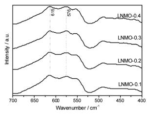
Fig. 2 FT-IR spectra of  $LiNi_{0.5}Mn_{1.5}O_4$  samples synthesized at different reactant concentrations.
