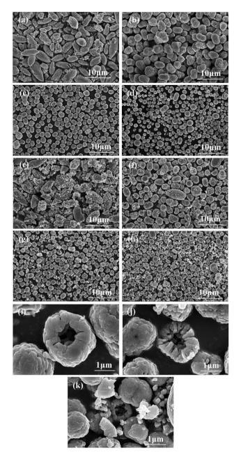
Fig. 3 SEM images of carbonate precursor (a–d) and LiNi $_{0.5}$ Mn $_{1.5}$ O $_4$  samples (e–k) (a and e) 0.1 mol L<sup>-1</sup>, (b, f and i) 0.2 mol L<sup>-1</sup>, (c, g and j) 0.3 mol L<sup>-1</sup>, (d, h and k) 0.4 mol L<sup>-1</sup>.
