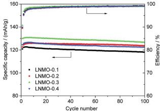
Fig. 6 Cycling performance and coulombic efficiency of LiNi $_{0.5}$ -Mn $_{1.5}$ O $_{4}$  samples synthesized at different reactant concentrations at 1C rate.
