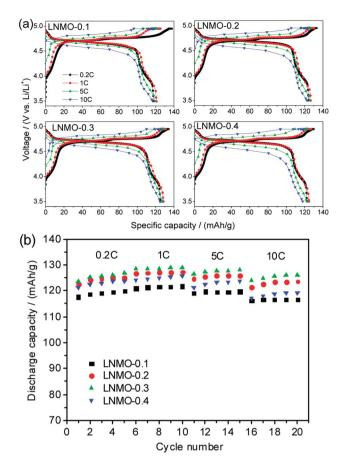
Fig. 4 Charge/discharge curves at various rates (a) and rate capability curves (b) for  $\text{LiNi}_{0.5}\text{Mn}_{1.5}\text{O}_4$  samples synthesized at different reactant concentrations.
