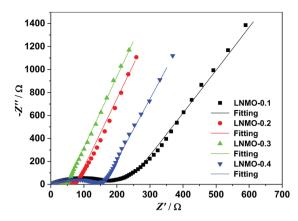
Fig. 7 Nyquist plots for LiNi<sub>0.5</sub>Mn<sub>1.5</sub>O<sub>4</sub> samples synthesized at different reactant concentrations.
