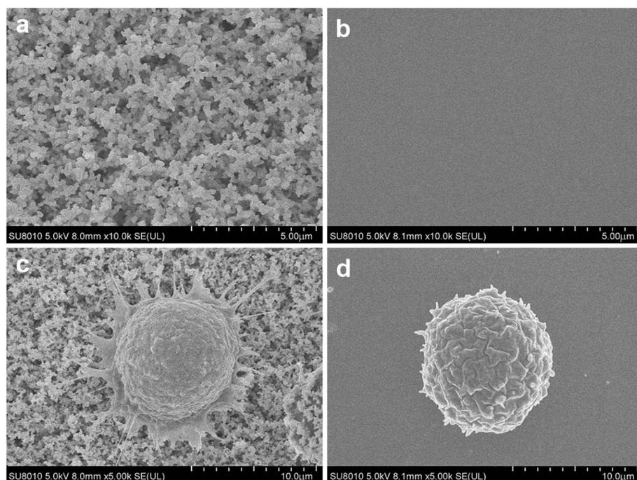
Fig. 2 (a) The scanning electron microscope (SEM) image of nanodendritic surface. (b) Flat glass surface without nanostructure. (c) A captured cell with many filopodia protruded on the nanobiointerface chip. (d) A captured cell with regular spherical shape on the flat glass chip.
