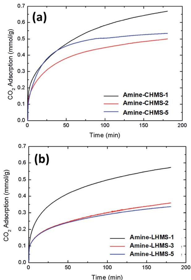
Fig. 13 Selective gas uptake of CO<sub>2</sub> calibrated by subtracting N<sub>2</sub> gas uptake for all amine-modified samples. (a) Amine-CHMS and (b) amine-LHMS samples.
