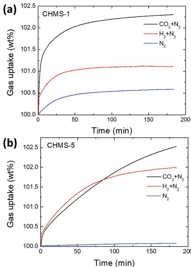
Fig. 9 Selective CO<sub>2</sub> and H<sub>2</sub> gas uptake of pure CHMS samples at 25 °C and 1 atm. Gas uptakes under mixed flows of CO<sub>2</sub> + N<sub>2</sub> gases, H<sub>2</sub> + N<sub>2</sub> gases and pure N<sub>2</sub> gas for (a) CHMS-1 and (b) CHMS-5 samples.
