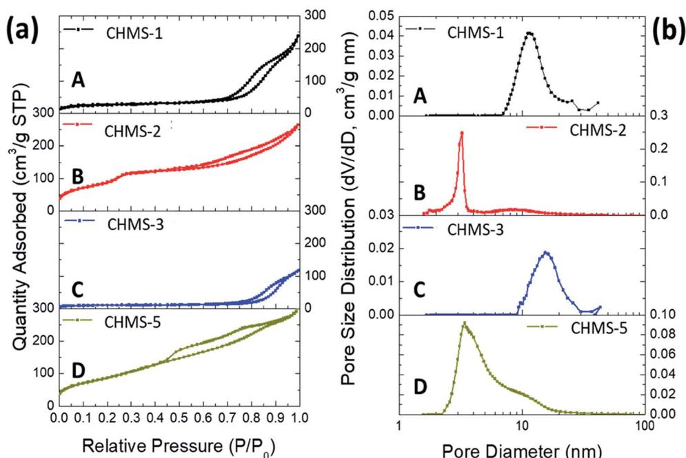
Fig. 7 (a) N<sub>2</sub> adsorption–desorption isotherms for (A) CHMS-1, (B) CHMS-2, (C) CHMS-3, and (D) CHMS-5 samples. (b) Corresponding pore size distribution (PSD) curves of the samples for (A) CHMS-1, (B) CHMS-2, (C) CHMS-3, and (D) CHMS-5 obtained by KJS method.
