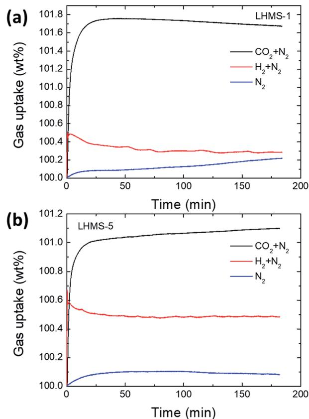
Fig. 10 Selective CO<sub>2</sub> and H<sub>2</sub> gas uptake of pure LHMS samples at 25 °C and 1 atm. Gas uptakes under mixed flows of CO<sub>2</sub> + N<sub>2</sub> gases, H<sub>2</sub> + N<sub>2</sub> gases and pure N<sub>2</sub> gas for (a) LHMS-1 and (b) LHMS-5 samples.
