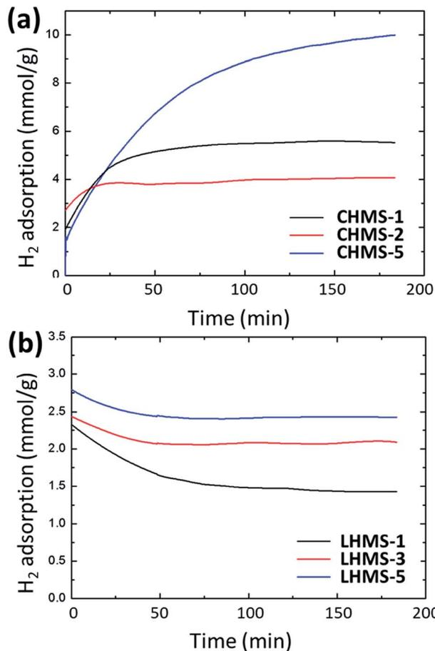
Fig. 11 Selective gas uptake of H<sub>2</sub> calibrated by subtracting N<sub>2</sub> gas uptake for (a) CHMS and (b) LHMS samples.
