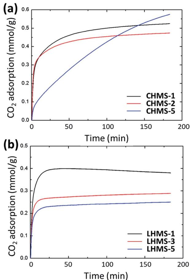
Fig. 12 Selective gas uptake of CO<sub>2</sub> calibrated by subtracting N<sub>2</sub> gas uptake for (a) CHMS and (b) LHMS samples.
