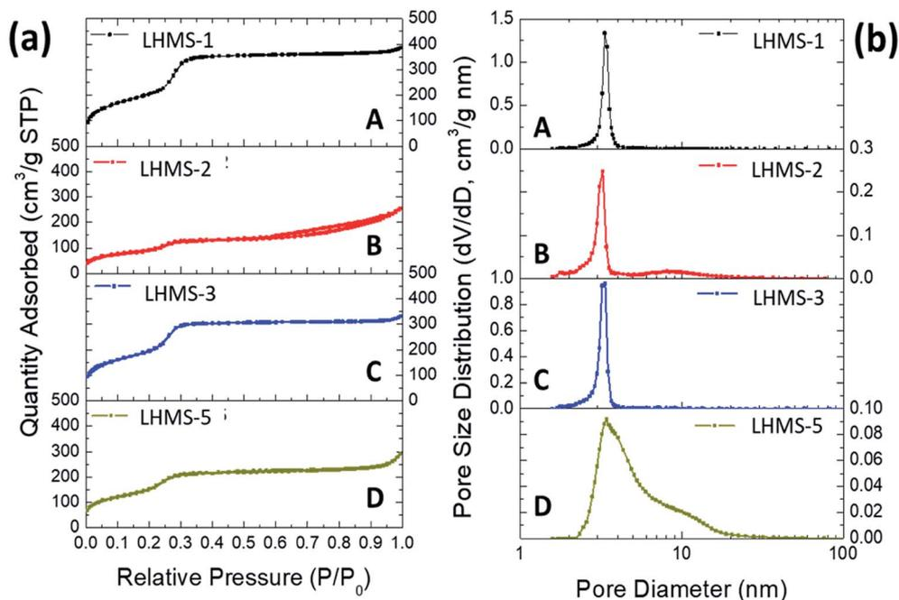
Fig. 8 (a) N<sub>2</sub> adsorption-desorption isotherms for (A) LHMS-1, (B) LHMS-2, (C) LHMS-3, and (D) LHMS-5 samples. (b) Corresponding pore size distribution (PSD) curves of the samples for (A) LHMS-1, (B) LHMS-2, (C) LHMS-3, and (D) LHMS-5 obtained by KJS method.
