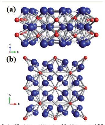
Fig. 1 (a) Front view and (b) top view of the I4/m structure of  $W_2B$  under ambient pressure. Large blue and small red spheres represent tungsten and boron atoms, respectively.
