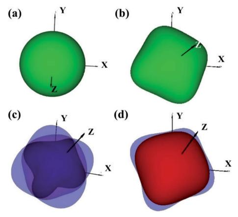
Fig. 5 3D representations of elastic properties based on theoretical elastic stiffness constants  $C_{ij}$  of  $W_2B$  at a small strain of 0.3% (near the equilibrium). (a) Uniaxial compression modulus representation surfaces. (b) Young's modulus E representation surfaces. (c) Poisson's ratio v representation surfaces. (d) Shear modulus E representation surfaces.
