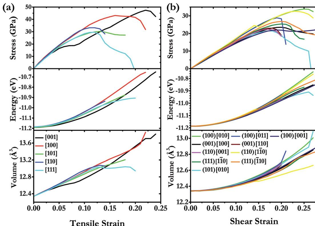
Fig. 6 (a) Calculated stress responses under tensile strain in various deformation directions and (b) calculated stress–strain curves on various shear sliding planes in different directions under pure shear deformation for  $W_2B$  at large strain under ambient pressure.
