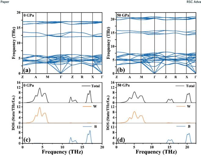
(a and b) Calculated phonon dispersion curves and (c and d) phonon density of states for W₂B at 0 GPa and 50 GPa, respectively
