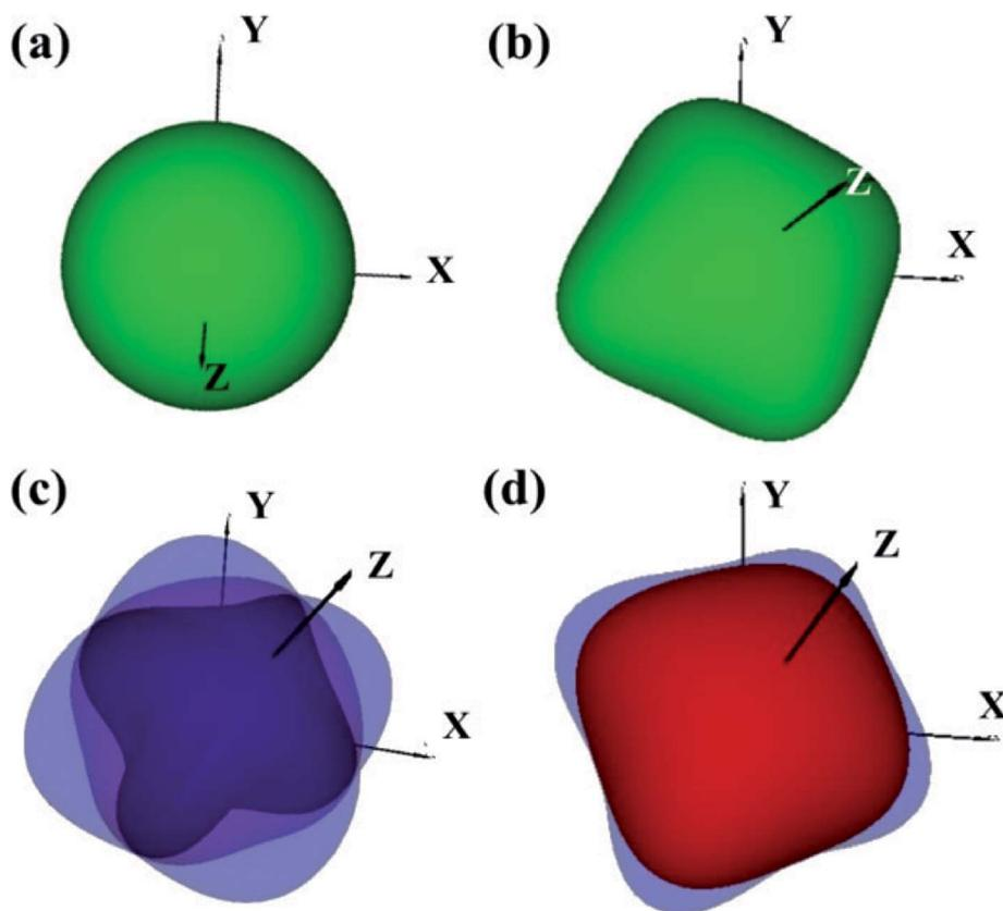
Fig. 5 3D representations of elastic properties based on theoretical elastic stiffness constants  $C_{ij}$  of  $W_2B$  at a small strain of 0.3% (near the equilibrium). (a) Uniaxial compression modulus representation surfaces. (b) Young's modulus  $E$  representation surfaces. (c) Poisson's ratio  $\nu$  representation surfaces. (d) Shear modulus  $G$  representation surfaces.
