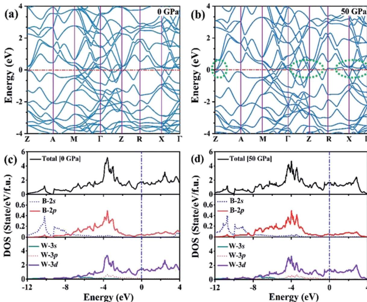
Fig. 3 (a and b) Electronic band structures and (c and d) electronic total and partial DOS of the  $W_2B$  at 0 GPa and 50 GPa, respectively. The zero of the energy coincides with the Fermi level. The green dashed circles highlight the changes of electronic band structures near the Fermi level.
