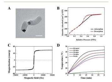
Fig. 1 Characterization of Janus M-MSNs: (A) TEM, (B)  $N_2$  sorption isotherms of Janus M-MSNs, (C) magnetization curves, (D) temperature—time curves of Janus M-MSNs suspensions at various concentrations under ACMF exposure.
