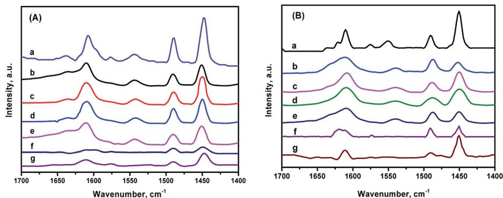
Fig. 9 Pyridine-FTIR spectra of different catalysts: (a)  $\text{NiMo}/\text{ZSM-5}$ , (b)  $\text{NiMo}/\text{ZK-1}$  (c)  $\text{NiMo}/\text{ZK-2}$ , (d)  $\text{NiMo}/\text{ZK-3}$ , (e)  $\text{NiMo}/\text{ZK-4}$ , (f)  $\text{NiMo}/\text{KIT-6}$ , (g)  $\text{NiMo}/\text{Al}_2\text{O}_3$  after degassing at 473 K (A) and 623 K (B).
