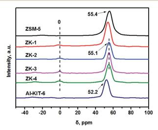
Fig. 5 <sup>27</sup>Al MAS NMR spectra of the as-synthesized materials.
