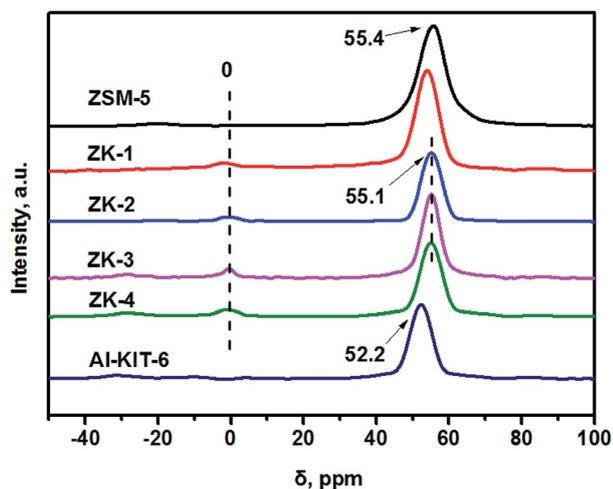
Fig. 5  $^{27}\text{Al}$  MAS NMR spectra of the as-synthesized materials.
