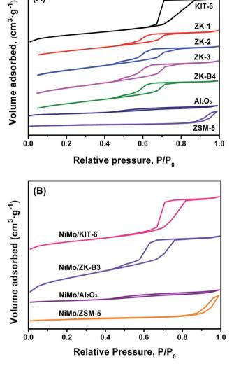
Fig. 7 N<sub>2</sub> adsorption-desorption isotherms of the as-synthesized materials (A) and corresponding catalysts (B).
