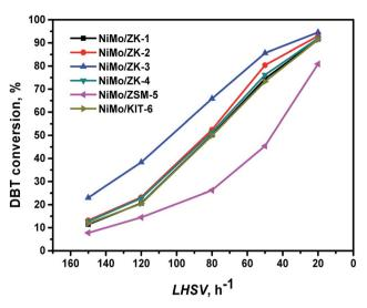
Fig. 13 DBT conversions of different NiMo-supported catalysts in the HDS reaction.
