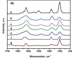
Fig. 9 Pyridine-FTIR spectra of different catalysts: (a) NiMo/ZSM-5, (b) NiMo/ZK-1 (c) NiMo/ZK-2, (d) NiMo/ZK-3, (e) NiMo/ZK-4, (f) NiMo/KIT-6, (g) NiMo/Al<sub>2</sub>O<sub>3</sub> after degassing at 473 K (A) and 623 K (B).
