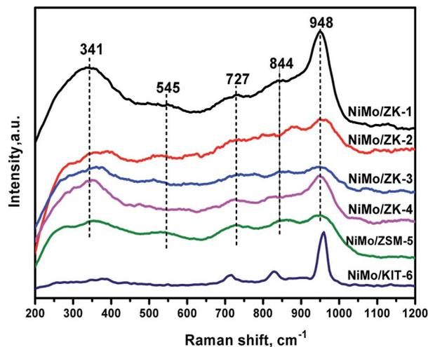
Fig. 11 Raman spectra of the different catalysts.
