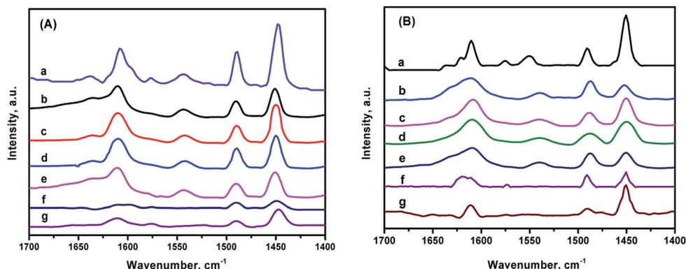
Fig. 9 Pyridine-FTIR spectra of different catalysts: (a) NiMo/ZSM-5, (b) NiMo/ZK-1 (c) NiMo/ZK-2, (d) NiMo/ZK-3, (e) NiMo/ZK-4, (f) NiMo/KIT-6, (g) NiMo/ $\text{Al}_2\text{O}_3$  after degassing at 473 K (A) and 623 K (B).
