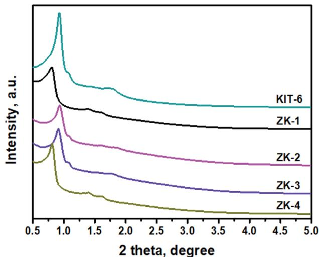
Fig. 3 Small-angle XRD patterns of the different materials.
