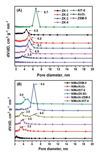
Fig. 8 Pore size distribution of the different supports (A) and corresponding catalysts (B).
