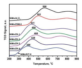
Fig. 10 H<sub>2</sub>-TPR curves of the supported NiMo catalysts.
