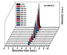
Fig. 5 HPLC spectra of benzotriazole degradation by (a) BiOI-C and (b) BiOI-G.
