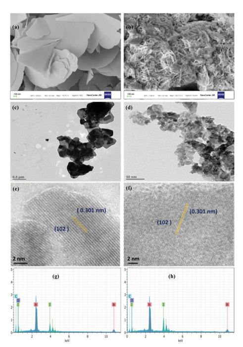
Fig. 2 (a and b) FESEM images, (c and d) TEM images, (e and f) HR-TEM images, (g and h) EDS images of BiOI-C (left) and BiOI-G (right).
