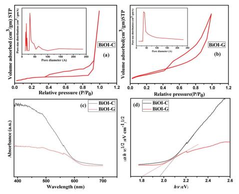
Fig. 3 (a and b)  $N_2$  adsorption—desorption isotherms and pore size distributions, (c and d) UV-Vis DRS and plot of  $(\alpha h \nu)^n$  vs.  $h\nu$  of BiOI-C and BiOI-G
