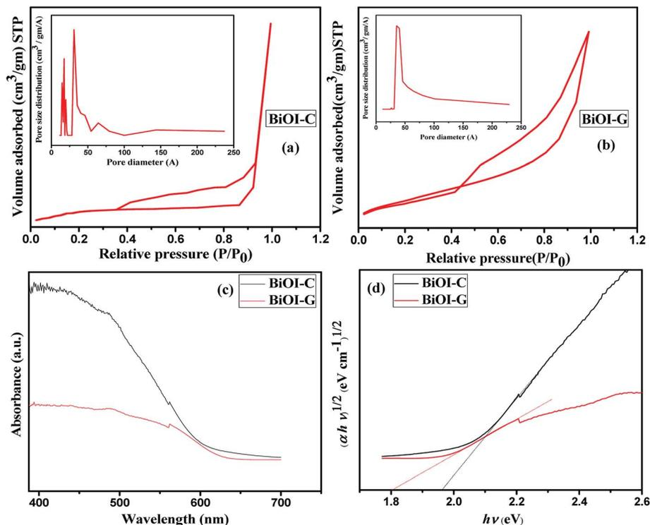
Fig. 3 (a and b) N<sub>2</sub> adsorption–desorption isotherms and pore size distributions, (c and d) UV-Vis DRS and plot of  $(\alpha h\nu)^{1/2}$  vs.  $h\nu$  of BiOI-C and BiOI-G.
