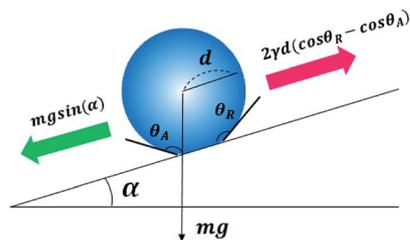
Fig. 9 Schematic view of water droplet on a tilted surface.
