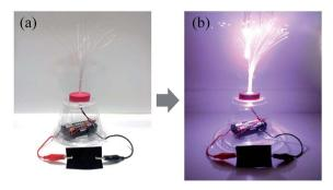
Fig. 4 Photos of LED lamps connected to the polypyrrole deposited and hydrophobic coated cotton fabric.
