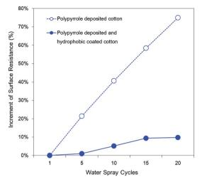
Fig. 14 Effect of moisture on the surface resistivity of the cotton fabrics treated with polypyrrole deposition and hydrophobic coating.
