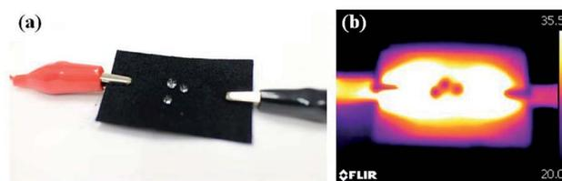
Fig. 7 The photo (a) and infrared thermal image (b) of sample with electro heating effect and superhydrophobicity.
