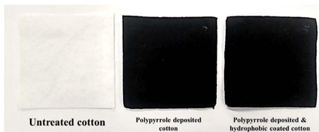
Fig. 2 Photo of polypyrrole deposited cotton samples.
