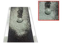
Fig. 10 Photos of the polypyrrole deposited and hydrophobic coated cotton fabric after scattering silicon carbide particles on the surface and cleaning with water droplet.
