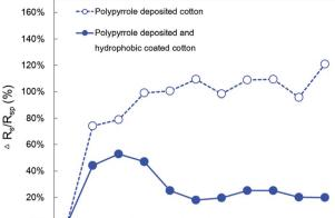
Fig. 11 Effect of atmospheric ageing on the surface resistivity of cotton fabrics treated with polypyrrole deposition and hydrophobic
