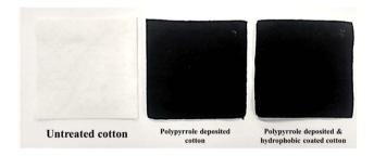
Fig. 2 Photo of polypyrrole deposited cotton samples.
