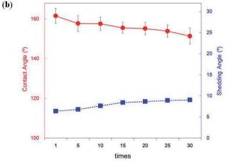
Fig. 12 The rubbing fastness (a), and contact angles and shedding angles (b) of the cotton fabrics treated with polypyrrole deposition and hydrophobic coating after testing with roll tape cleaner.
