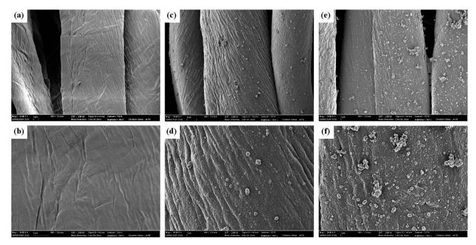
Fig. 3 SEM images of pristine cotton (a and b), polypyrrole deposited cotton (c and d) and polypyrrole deposited and hydrophobic coated cotton (e and f).
