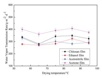
Fig. 8 Effect of drying temperature on water vapor permeability of chitosan membranes prepared from chitosan solution, and chitosan suspension using ethanol, acetonitrile, and acetone.
