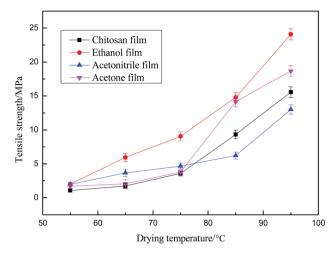
Fig. 6 Effect of drying temperature on tensile strength of membranes prepared from (a) chitosan solution, and chitosan suspension using (b) ethanol, (c) acetonitrile, and (d) acetone.
