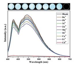
Fig. 4 Fluorescence responses of the complex with different toxic metal ions ( $1 \times 10^{-3}$  mol L<sup>-1</sup>, excited at 365 nm).
