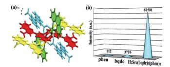
Fig. 2 (a) The crystal structure of the title complex. (b) The emission intensities of phen, bqdc and  $H_2Sr_2(bqdc)_3(phen)_2$ .
