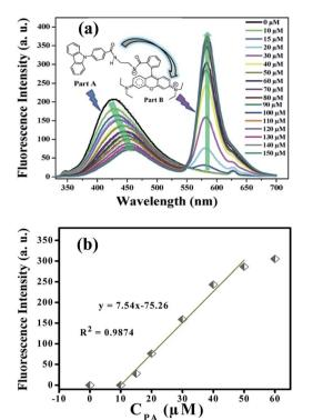
Fig. 7 (a) Fluorescence response of L (20  $\mu$ M) upon addition of PA from 10 to150  $\mu$ M (inset, the proposed structure of the spiro-lactam ring-opening product); (b) linear fitting analysis ( $\lambda_{ex}=314$  nm,  $\lambda_{em}=586$  nm) of the fluorescence intensity at 586 nm *versus* the concentration of PA.
