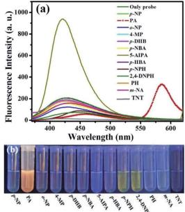
Fig. 4 (a) Fluorescence spectra of L (20  $\mu$ M) in the absence and presence of 200  $\mu$ M various aromatic compounds ( $\lambda_{ex}=314$  nm, slits: 2.5 nm/5 nm; slits: 1.0 nm/5 nm for 5-AlPA); (b) photograph of probe solutions with different aromatic compounds under 365 nm UV lamp.
