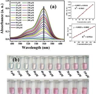
Fig. 6 (a) Absorption intensity of probe solution with various concentrations of PA (left) and linear fitting curve of the absorption intensity at 560 nm *versus* the concentration of PA (right); (b) color changes of the probe solutions with gradually addition of PA under visible light.
