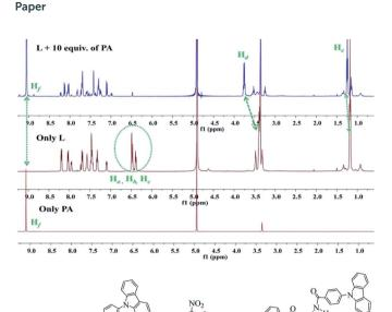
Fig. 9  $^{1}$ HNMR spectra of L, PA and the mixture of L + PA in CD<sub>3</sub>OD
