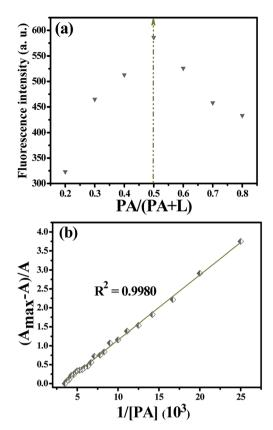
Fig. 8 (a) Job's plot of L + PA complex in ethanol. ( $\lambda_{ex} = 500$  nm,  $\lambda_{em} = 586$  nm, slits: 2.5 nm/5 nm); (b) Benesi–Hildebrand plot (absorbance at 560 nm) of probe L assuming a 1 : 1 binding stoichiometry with PA.
