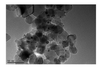
Fig. 2 TEM image of Au (1 wt%)-TiO<sub>2</sub>
