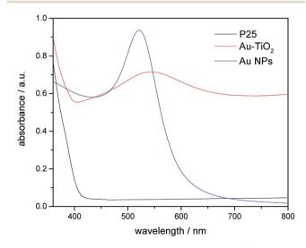
Fig. 3 Diffuse-reflectance UV-Vis spectra of bare  ${\rm TiO_2}$  (black), Au NPs (blue) and  ${\rm Au-TiO_2}$  (red).
