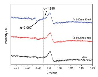
Fig. 5 EPR spectra of Au-TiO<sub>2</sub> obtained in the dark and under visible light illumination (≥500 nm) at 90 K.
