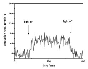
Fig. 4 Photocatalytic H<sub>2</sub> evolution rate of Au-TiO<sub>2</sub> obtained from CH<sub>3</sub>OH/H<sub>2</sub>O mixtures upon visible light illumination in the presence of a 500 nm cutoff filter.
