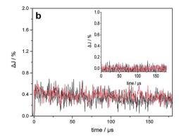
Fig. 6 (a) Transient absorption signals of bare  $TiO_2$  observed at 680 nm upon 420 nm laser excitation; (b) transient absorption signals of bare  $TiO_2$  (inset) and  $Au-TiO_2$  observed at 680 nm (black) and 400 nm (red) upon 532 nm laser excitation in a  $N_2$  atmosphere.
