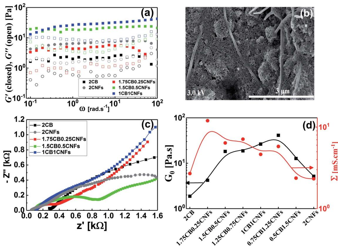
Fig. 8 (a) Dynamic frequency sweep, (b) scanning electron micrograph, (c) impedance spectra (Nyquist plots), and (d) variation of plateau modulus ( $G_0$ ) and electrical conductivity ( $\Sigma$ ) for hybrid carbon materials. The concentration of carbon materials is represented by wt% (e.g. 2CB, and 1.75CB0.25CNFs denote, respectively, 2.0 wt% CB, and 1.75 wt% CB + 0.25 wt% CNFs, etc.).
