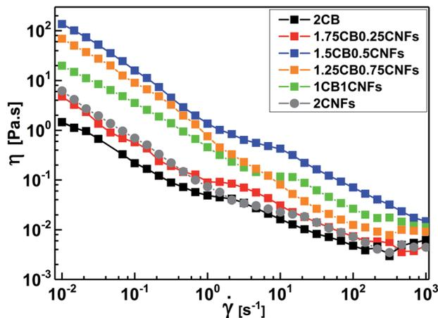
Fig. 9 Variation of steady-shear viscosity ( $\eta$ ) with shear rate  $\dot{\gamma}$  for aqueous dispersions of 2.0 wt% CB (2CB), 2.0 wt% CNFs (2CNFs), and some selected hybrid dispersions (e.g. 1.75KB0.25CNFs denotes 1.75 wt% CB + 0.25 wt% CNFs).
