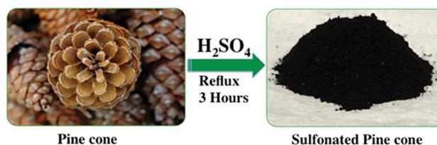
Scheme 1 Preparation of sulfonated pine cone (PC-SO<sub>3</sub>H).
