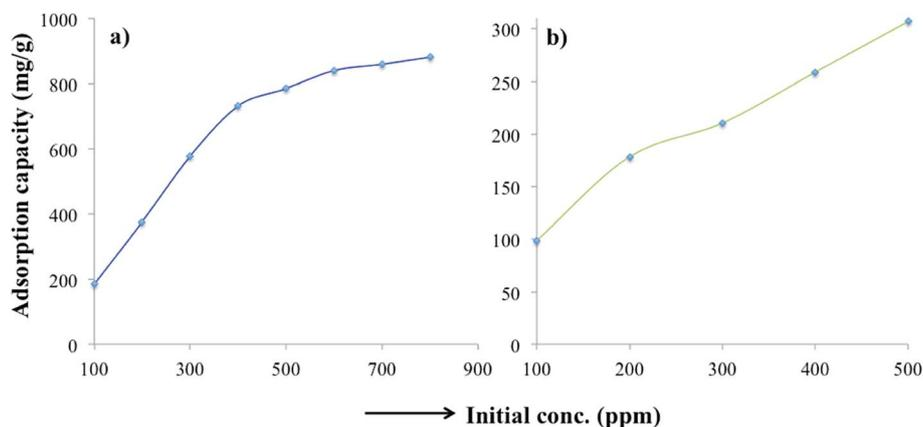
Fig. 11 Adsorption capacity of PC-SO<sub>3</sub>H for (a) MB and (b) TC from tap water matrix. Initial MB concentration = 100–800 mg L<sup>-1</sup>,  $V = 20$  mL and adsorbent = 10 mg; initial TC concentration = 100–500 mg L<sup>-1</sup>,  $V = 20$  mL and adsorbent = 20 mg.
