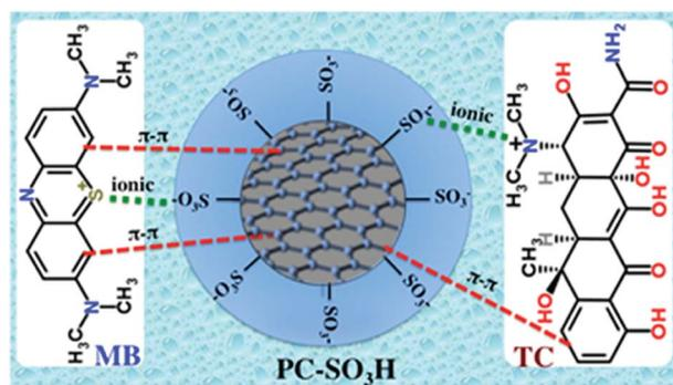
Scheme 3 Proposed adsorption mechanism of the PC-SO<sub>3</sub>H towards the MB and TC.
