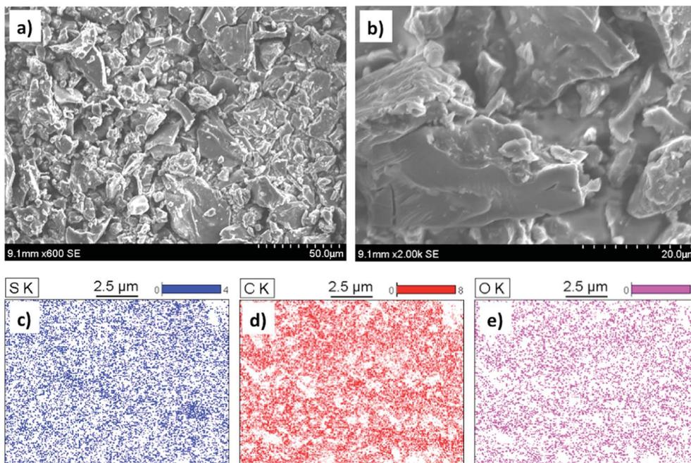
Fig. 1 (a and b) SEM images of the PC-SO<sub>3</sub>H with varying magnifications and (c–e) elemental mapping images of the PC-SO<sub>3</sub>H depicting the presence of sulfur, carbon and the oxygen.
