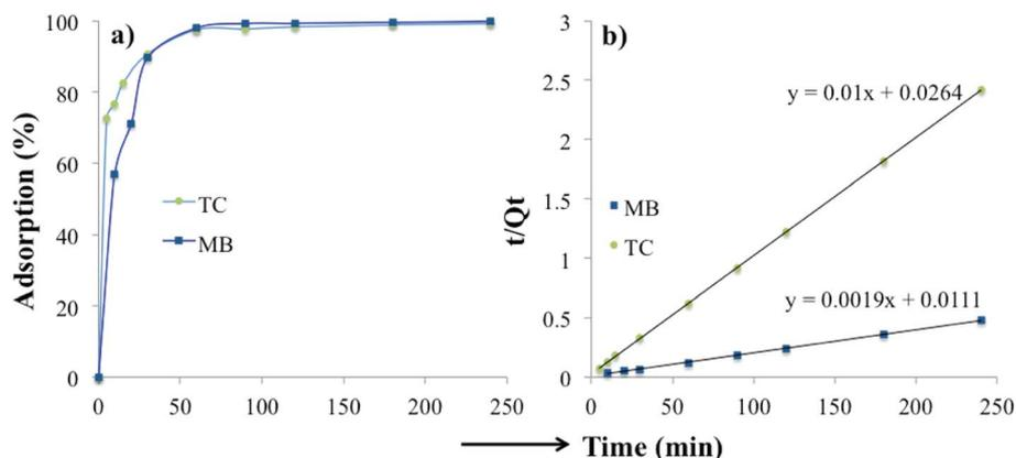
Fig. 8 (a) Time-dependent percent adsorption of MB and TC and (b) the corresponding pseudo-second-order kinetics adsorption. Initial MB concentration = 200 mg L<sup>-1</sup>, V = 40 mL and adsorbent = 20 mg; initial TC concentration = 50 ppm, V = 20 mL and adsorbent = 10 mg.
