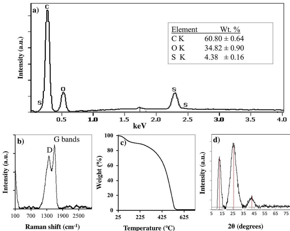
Fig. 2 (a) EDS spectra showing the elemental composition, (b) Raman spectra shows the carbonaceous nature (c) the thermal gravimetric curve depicts the thermal stability and (d) XRPD pattern shows the crystalline carbonaceous nature of the PC-SO<sub>3</sub>H.
