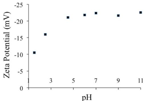
Fig. 5 pH-dependent zeta potential of the PC-SO<sub>3</sub>H in water.
