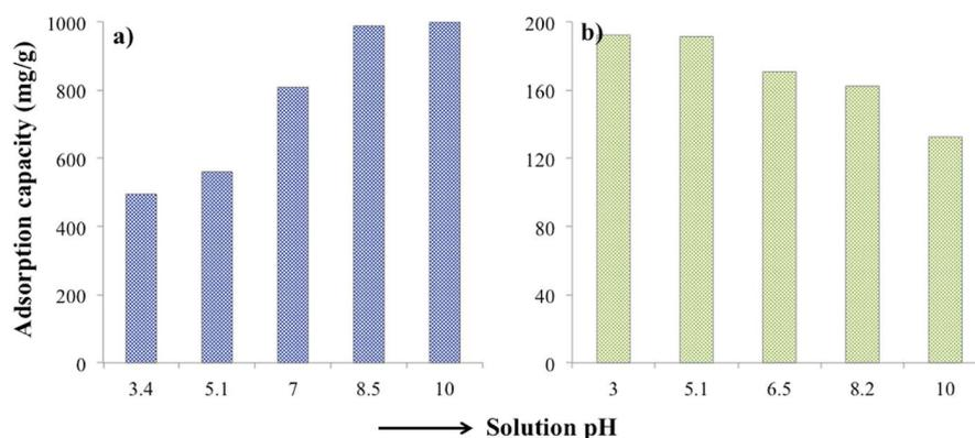
Fig. 6 pH dependent adsorption of (a) MB and (b) TC by PC-SO<sub>3</sub>H, respectively. Initial MB concentration = 1000 mg L<sup>-1</sup>,  $V = 20$  mL and adsorbent = 20 mg; initial TC concentration = 200 mg L<sup>-1</sup>,  $V = 20$  mL and adsorbent = 20 mg.
