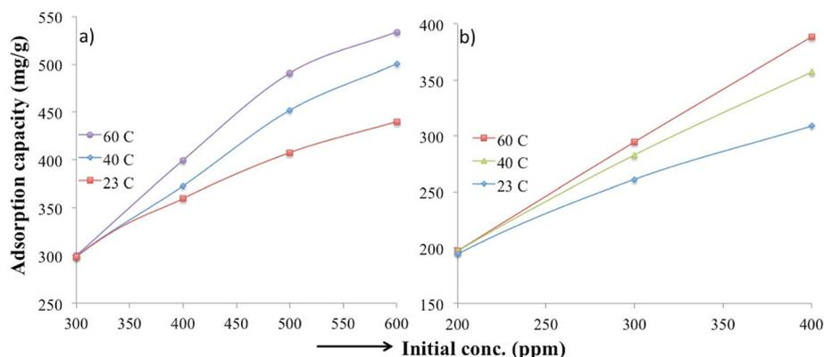
Fig. 9 Temperature-dependent adsorption capacities of the PC-SO<sub>3</sub>H for (a) MB and (b) TC at pH 3.25 and 3.75, respectively.
