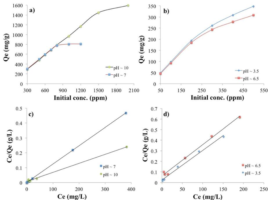
Fig. 7 Adsorption capacity of PC-SO<sub>3</sub>H towards (a) MB and (b) TC at different initial pollutant concentrations and pH. Corresponding Langmuir isotherm models for the adsorption of (c) MB and (d) TC onto PC-SO<sub>3</sub>H.
