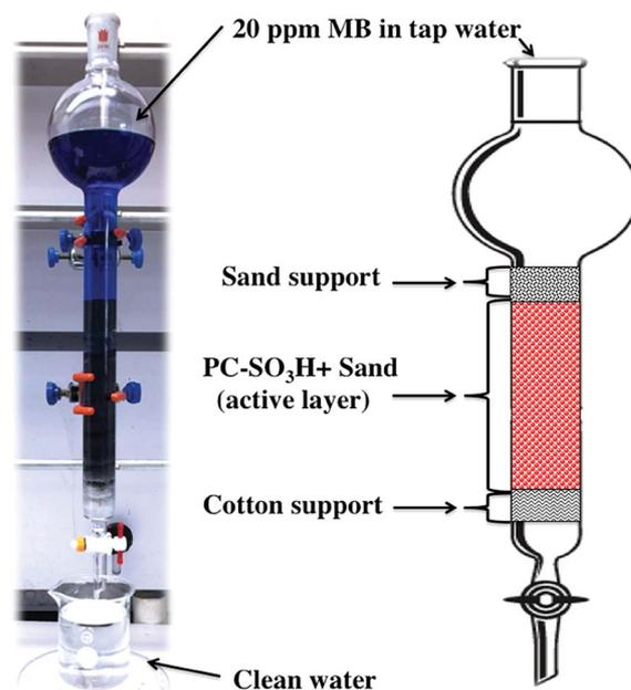
Scheme 2 Design of the column filter packed with PC-SO<sub>3</sub>H and sand for the continuous adsorption of MB.
