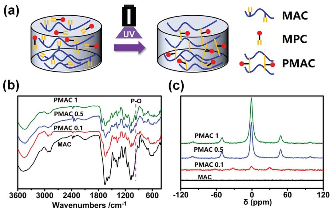
Fig. 2 The schematic of preparation process and characterization of PMAC. (a) Diagrammatic sketch of reaction of PMAC; (b) FTIR result of MAC and different PMAC groups; (c)  $^{31}\text{P}$  NMR of MAC and different PMAC groups.
