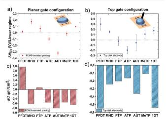
Fig. 4 Threshold voltage shifts extracted from transfer characteristic in linear regime ( $V_{\rm DS}=-0.1$  V) and the corresponding capacitance shifts calculated according to eqn (2); The EGOFETs are measured by means of (a) and (c) the planar gate functionalized with SAMs by PDMS-assisted printing and (b) and (d) by using a gold disk electrode functionalized with a standard protocol.
