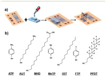
Fig. 2 (a) Schematic diagram of PDMS-assisted printing of selfassembled monolayers. (b) Molecular structure of the SAMs subject of this study.
