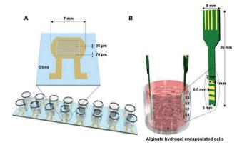
Fig. 1 (A) A 2D impedance cell sensor array composed of 16 sensors with a pair of interdigitated electrodes and (B) a 3D impedance cell sensor consisting of four pairs of vertically aligned electrodes.
