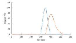
Fig. 5 Laser scattering graph of the urea-DMG-C $_{60}$  system, (a): 0.45 mol L $^{-1}$  of HCl + 1.65  $\times$  10 $^{-3}$  mol L $^{-1}$  of TSC + 3.2 mmol L $^{-1}$  of DMG + 0.056 mmol L $^{-1}$  of C $_{60}$ ; (b): a + 166.5 nmol L $^{-1}$  of urea.
