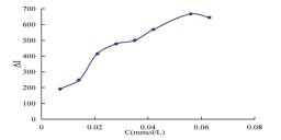
Fig. 9 Effect of  $C_{60}$  concentration, 133.20 nmol  $L^{-1}$  of urea + 0.45 mol  $L^{-1}$  of HCl + 1.65 mmol  $L^{-1}$  of TSC + 3.2 mmol  $L^{-1}$  of DMG +  $C_{60}$ .
