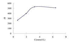
Fig. 8 Effect of DMG concentration, 133.20 nmol  $L^{-1}$  of urea + 0.45 mol  $L^{-1}$  of HCl + 1.65 mmol  $L^{-1}$  of TSC + DMG + 0.056 mmol  $L^{-1}$  of C<sub>60</sub>.
