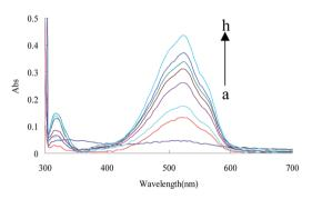
Fig. 3 Absorption spectra of the urea-DMG- $C_{60}$  system, (a) 0.45 mol  $L^{-1}$  of HCl + 1.65 ×  $10^{-3}$  mol  $L^{-1}$  of TSC + 3.2 mmol  $L^{-1}$  of DMG + 0.056 mmol  $L^{-1}$  of  $C_{60}$ ; (b) a + 16.65 nmol  $L^{-1}$  of urea; (c): a + 66.60 nmol  $L^{-1}$  of urea; (d): a + 133.20 nmol  $L^{-1}$  of urea; (e): a + 233.10 nmol  $L^{-1}$  of urea; (f): a + 399.6 nmol  $L^{-1}$  of urea; (g): a + 499.50 nmol  $L^{-1}$  of urea; (h): a + 666.0 nmol  $L^{-1}$  of urea.
