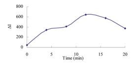
Fig. 11 Effect of bath time 133.20 nmol L $^{-1}$  of urea + 0.45 mol L $^{-1}$  of HCl + 1.65 mmol L $^{-1}$  of TSC + 3.2 mmol L $^{-1}$  of DMG + 0.056 mmol L $^{-1}$  of C<sub>60</sub>.
