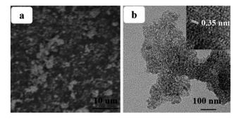
Fig. 9 SEM (a) and TEM (b) images of the RGO-TiO<sub>2</sub> scattering layer, the high magnificent image of the material is shown in the inset.
