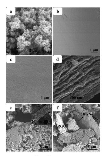
Fig. 1 SEM images of (a)  $TiO_2$  (b) transport layer with the RGO as the terminal layer (c) transport layer with the  $TiO_2$  as the terminal layer (d) cross-section view of the transport layer (e) the 3DGNs added work layer (the original 3DGNs shown in the inset) (f) the 3DGNs and RGO co-modified work layer.
