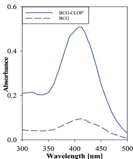
Fig. 7 Absorption spectrum of 1.0 mmol L<sup>-1</sup> CLOP·H<sub>2</sub>SO<sub>4</sub> with 1.0 mmol L<sup>-1</sup> BCG against a blank and 1.0 mmol L<sup>-1</sup> BCG against chloroform as a blank.
