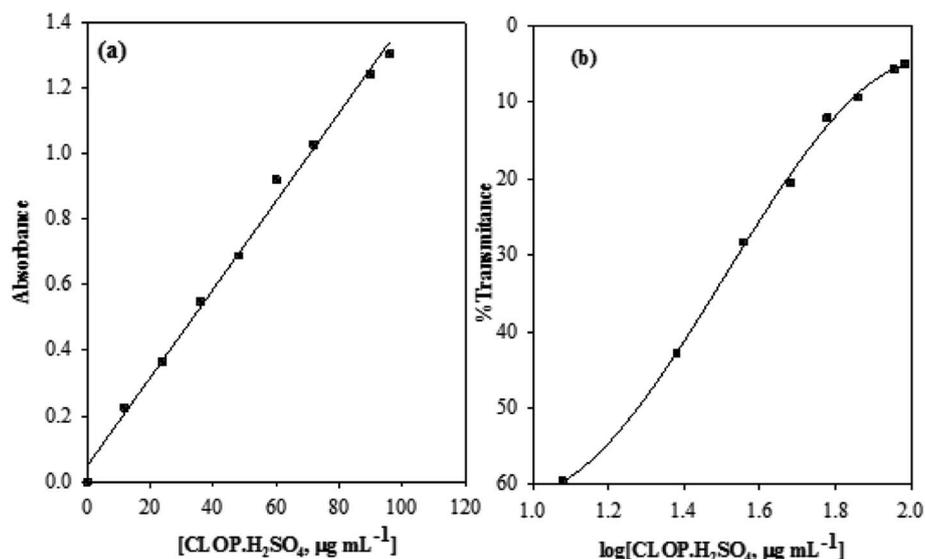
**Fig. 10** Calibration curve (a) and Ringbom plot (b) for the determination of CLOP·H<sub>2</sub>SO<sub>4</sub> with BCG.
