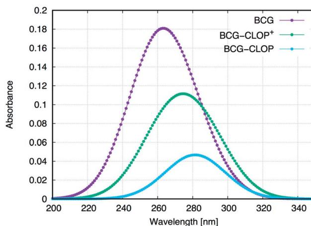
Fig. 6 Calculated UV-visible spectra for BCG and its ion-pairs with CLOP and CLOP<sup>+</sup> at the B3LYP/6-31+G(d,p) + Lan12dz level of theory and using CPCM.
