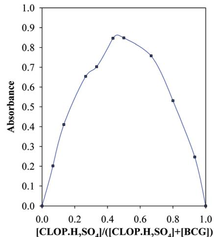
Fig. 8 Job's method of continuous variation for BCG–CLOP<sup>+</sup> ion pair.
