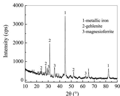
Fig. 2 XRD pattern of fabricated  $\text{Fe}^0/\text{C}$  ceramsites.
