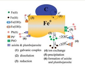
Fig. 10 Proposed mechanism in removing Pb( $_{\rm II}$ ) ions from aqueous solution by Fe $^{\rm 0}$ /C ceramsites.
