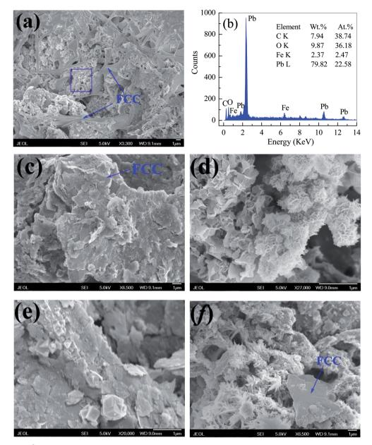
ig. 9 SEM images of  $Fe^0/C$  ceramsites after the Pb(ii) removal for 12 days and the EDX spectrum at selected area
