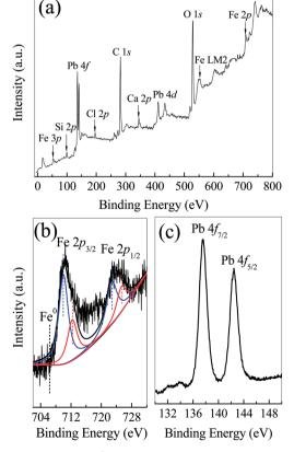
Fig. 8 XPS analysis of  ${\rm Fe^0/C}$  ceramsites in the removal of Pb(II) ions after 12 days: wide-scan survey (a) and high-resolution XPS lines of Fe 2p (b) and Pb 4f (c).
