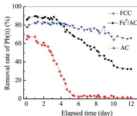
Fig. 6 Variation of removal rate of Pb(II) ions with elapsed time by Fe<sup>0</sup>/C ceramsites (FCC), Fe<sup>0</sup> powders/activated carbon (Fe<sup>0</sup>/AC) and activated carbon (AC).
