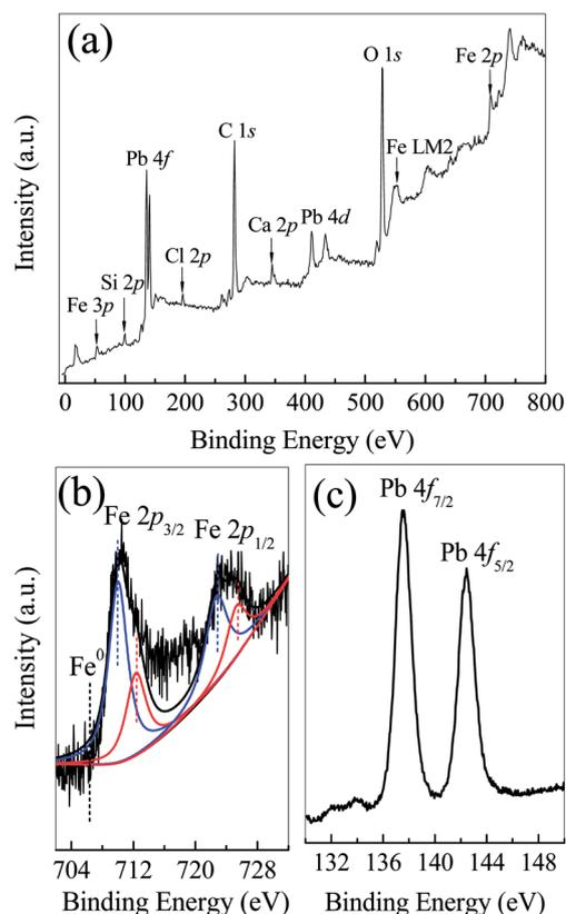
Fig. 8 XPS analysis of Fe<sup>0</sup>/C ceramsites in the removal of Pb(II) ions after 12 days: wide-scan survey (a) and high-resolution XPS lines of Fe 2p (b) and Pb 4f (c).
