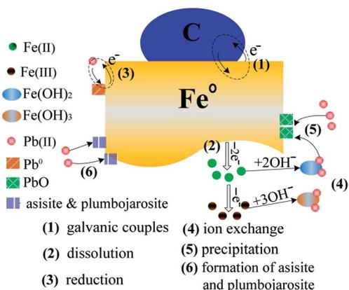
Fig. 10 Proposed mechanism in removing Pb(II) ions from aqueous solution by Fe<sup>0</sup>/C ceramsites.
