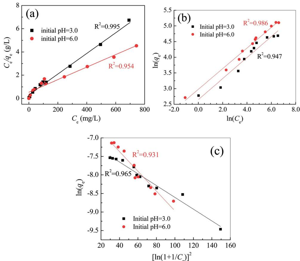
Fig. 5 Linearized fitting of Langmuir (a), Freundlich (b) and Dubinin–Raduskevich (c) isotherms for the Pb(II) removal by Fe<sup>0</sup>/C ceramsites at 25 °C.
