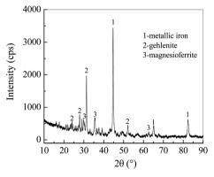
Fig. 2 XRD pattern of fabricated Fe<sup>0</sup>/C ceramsites.
