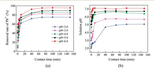
Fig. 4 Effect of initial pH on the Pb( $\pi$ ) removal by Fe<sup>0</sup>/C ceramsites (a) and variation of solution pH with contact time (b).
