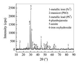
Fig. 7  $\,$  XRD pattern of Fe $^{0}$ /C ceramsites in the removal of Pb(II) ions after 12 days.
