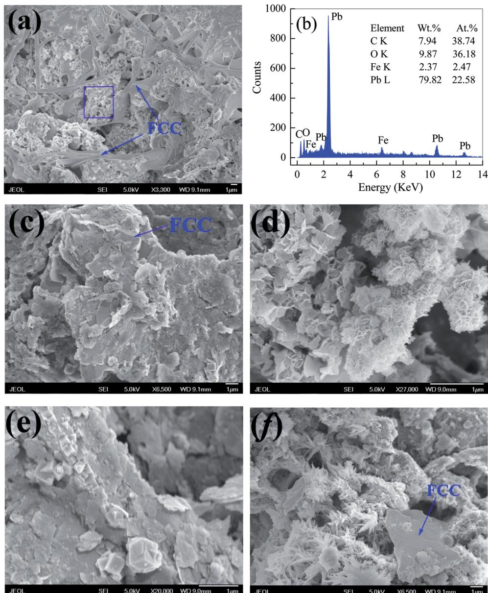
Fig. 9 SEM images of Fe<sup>0</sup>/C ceramsites after the Pb(II) removal for 12 days and the EDX spectrum at selected area.
