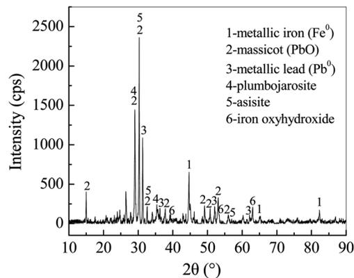
Fig. 7 XRD pattern of Fe<sup>0</sup>/C ceramsites in the removal of Pb(II) ions after 12 days.
