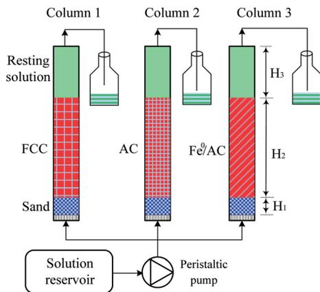
Fig. 1 Schematic diagram of column experiment design.
