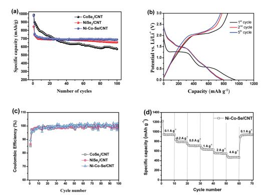
Fig. 5 (a) Comparison of the cycling performances of the  $CoSe_2/CNT$ ,  $NiSe_2/CNT$  and Ni-Co-Se/CNT during 100 cycles at a current density of 0.5 A  $g^{-1}$ . (b) Galvanostatic discharge/charge voltage profiles of the Ni-Co-Se/CNT composite at a current density of 0.2 A  $g^{-1}$ . (c) Coulombic efficiency at a current density of 0.2 A  $g^{-1}$ . (d) Rate performance of Ni-Co-Se/CNT.
