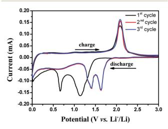
Fig. 4 Cyclic voltammogram profiles of the Ni–Co–Se/CNT composite with the scan rate of 0.1 mV  $\rm s^{-1}.$
