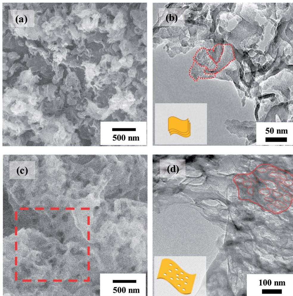
**Fig. 1** (a) SEM and (b) TEM images of g-C<sub>3</sub>N<sub>4</sub>. (c) SEM and (d) TEM images of P-g-C<sub>3</sub>N<sub>4</sub>. The selected region in red dashed square in (c) is enlarged and displayed in Fig. 4(a). The insets in (b) and (d) are schematic illustrations of overlapped nanosheets and porous sheet in the marked regions of g-C<sub>3</sub>N<sub>4</sub> and P-g-C<sub>3</sub>N<sub>4</sub>, respectively.
