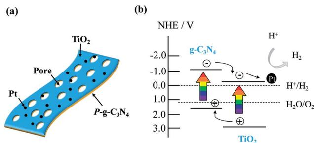
Fig. 11 (a) Schematic of Pt-loaded  $\text{TiO}_2@P\text{-}g\text{-C}_3\text{N}_4$  2D/2D hetero-junction structure. (b) Proposed mechanism of charge transfer for photocatalytic  $\text{H}_2$  evolution from Pt-loaded  $\text{TiO}_2@P\text{-}g\text{-C}_3\text{N}_4$ .
