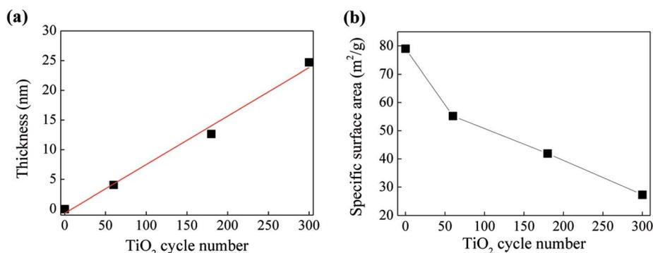
Fig. 6 Dependence of (a) thickness of TiO<sub>2</sub> and (b) specific surface area of the composites on TiO<sub>2</sub> cycle number.
