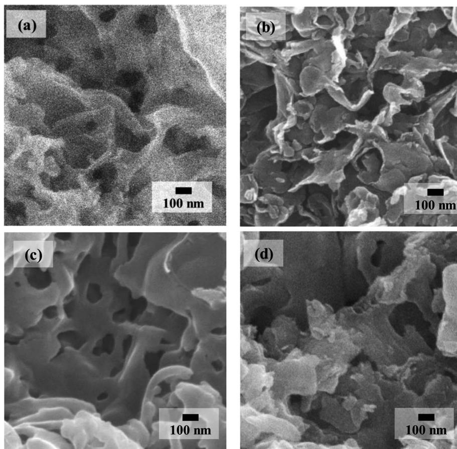
Fig. 4 SEM images of the samples. (a) As-prepared P-g-C<sub>3</sub>N<sub>4</sub> enlarged from Fig. 1(c). (b) Ti60–CN, (c) Ti180–CN, and (d) Ti300–CN. All composites were treated at 450 °C for 2 min by RTA in Ar.
