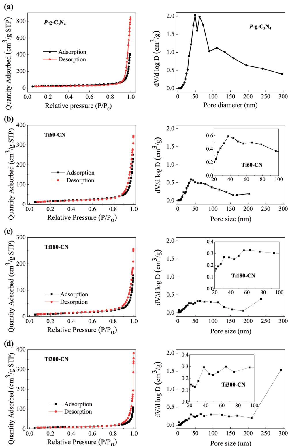
Fig. 7 Adsorption–desorption isotherms (left) and pore-size distributions (right) of (a) P-g-C<sub>3</sub>N<sub>4</sub>, (b) Ti60-CN, (c) Ti180-CN, and (d) Ti300-CN. The insets show the magnified pore size distributions in the range of 20–100 nm.
