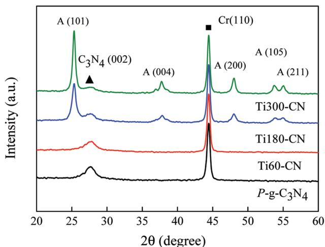
Fig. 3 XRD patterns of the samples. Cr is added as an internal standard, and the symbols of square (■) and triangle (▲) show the peak positions of Cr (110) and g-C<sub>3</sub>N<sub>4</sub> (002), respectively. The other diffraction peaks are ascribed to the anatase phase.
