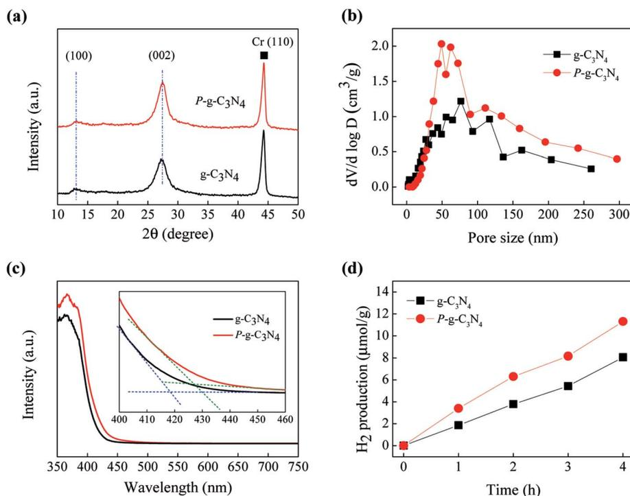
Fig. 2 Comparison between P-g-C<sub>3</sub>N<sub>4</sub> and g-C<sub>3</sub>N<sub>4</sub>. (a) XRD patterns, (b) pore size distributions, (c) UV-vis diffuse reflectance spectra, and (d) solar-driven H<sub>2</sub> evolution from 20 vol% methanol aqueous solution.
