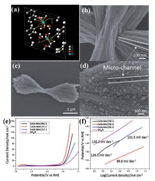
Fig. 7 (a) Crystallographic structure for the Co-MOF. Reproduced with permission from ref. 159. (b) FESEM images of the hybrid Co-Mo-MOF. (c and d) Carbonized product obtained by the pyrolysis of Co-Mo-MOF (e) LSV curves of different electrocatalysts at 1600 rpm (f) comparative Tafel slopes for the different carbonized products. Reproduced with permission from ref. 148. Copyright 2017 Wiley.
