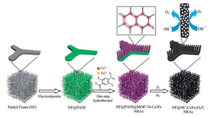
Fig. 8 Schematic representation of one-step PANI-assisted synthesis of a bimetal-organic framework NRAs and its derived porous  $CoFe_2O_4/C$  NRAs. Reproduced with permission from ref. 149. Copyright 2017 Wiley.
