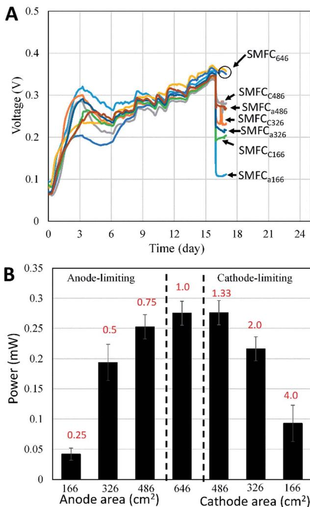
Fig. 2 Power generation of SMFCs with different electrode areas. (A) Voltage generation before and after cutting down electrode; (B) MP of different SMFCs, the red text indicate the SAR<sub>a/c</sub> of different SMFCs.
