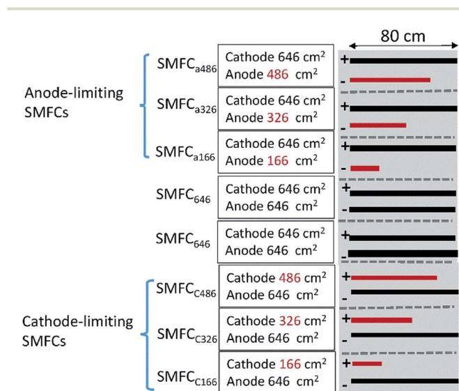
Fig. 1 Schematic of the SMFCs with different electrode surface areas and SAR<sub>a/c</sub>. “+” indicates cathode; “-” indicates anode; red bars indicate limiting electrodes.
