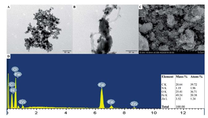
Fig. 3 TEM images of (A) Fe<sub>3</sub>O<sub>4</sub> and (B) Fe<sub>3</sub>O<sub>4</sub>/MWCNT@PDA. (C) SEM image and (D) EDS analysis of MMP/ZIF-8.
