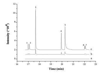
Fig. 6 TICs obtained by GC-MS/MS for the five triazole fungicides in real water samples obtained by the proposed method: river water spiked at (a) 0  $\mu$ g L<sup>-1</sup>, (b) 10  $\mu$ g L<sup>-1</sup>, and (c) 100  $\mu$ g L<sup>-1</sup>. Peak identification: (1) propiconazole-1, (2) propiconazole-2, (3) epoxiconazole, (4) fluquinconazole, (5) fenbuconazole, (6) difenoconazole-1, and (7) difenoconazole-2.
