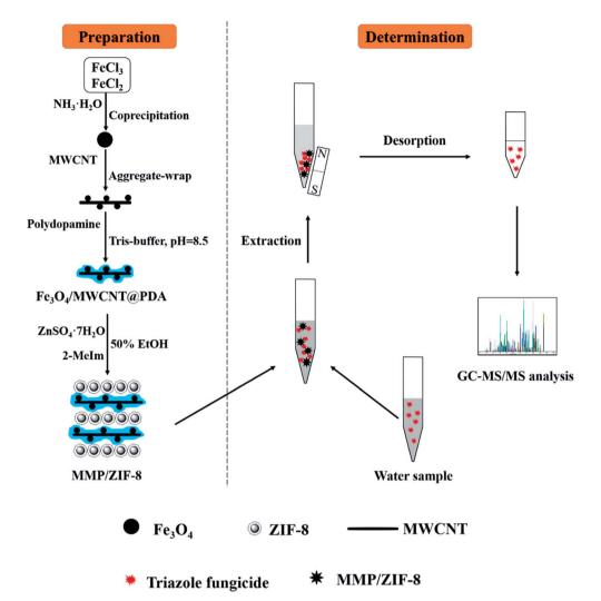
Fig. 1 Schematic diagram of the synthetic route to prepare MMP/ZIF-8 and the MSPE steps for triazole fungicide analysis.
