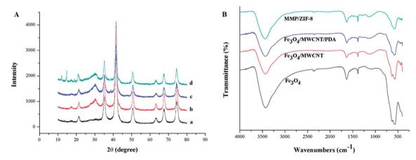
Fig. 2 (A) XRD patterns of (a) Fe<sub>3</sub>O<sub>4</sub>, (b) Fe<sub>3</sub>O<sub>4</sub>/MWCNTs, (c) Fe<sub>3</sub>O<sub>4</sub>/MWCNT@PDA, and (d) MMP/ZIF-8. (B) FT-IR spectra of the synthetic materials.
