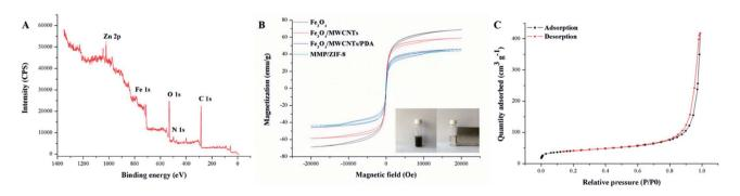
Fig. 4 (A) XPS spectra of MMP/ZIF-8; (B) magnetic curves of the synthetic materials; and (C) N₂ adsorption-desorption isotherms.
