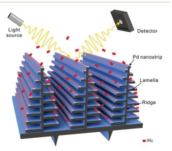
Fig. 1 Schematic illustration showing optical H<sub>2</sub> sensing based on the 3D heterogeneous structures that are consisted of Pd nanostrips and the photonic architectures of the Morpho butterfly wing scales.
