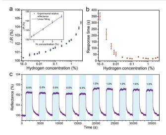
Fig. 5 Sensing performance of the Pd-modified Morpho butterfly scales to H<sub>2</sub>. (a) The plot showing relative reflectance at wavelength of 500 nm for different H2 concentrations. The inset figure shows a good linear relation between the relative reflectance and the H<sub>2</sub> concentration at the range of 0.75-4%. (b) The response time for different  $H_2$  concentrations. (c) Five cycles of H<sub>2</sub> exposure for concentrations of 0.5% and 1%.
