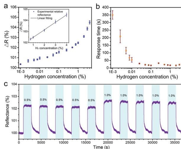
**Fig. 5** Sensing performance of the Pd-modified *Morpho* butterfly scales to H<sub>2</sub>. (a) The plot showing relative reflectance at wavelength of 500 nm for different H<sub>2</sub> concentrations. The inset figure shows a good linear relation between the relative reflectance and the H<sub>2</sub> concentration in the range of 0.75–4%. (b) The response time for different H<sub>2</sub> concentrations. (c) Five cycles of H<sub>2</sub> exposure for concentrations of 0.5% and 1%.
