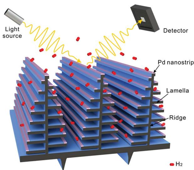
Fig. 1 Schematic illustration showing optical  $H_2$  sensing based on the 3D heterogeneous structures that are consisted of Pd nanostructures and the photonic architectures of the *Morpho* butterfly wing scales.
