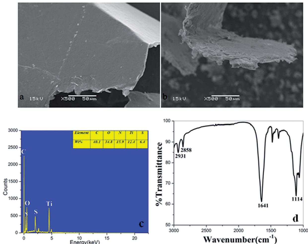
Fig. 2 SEM images of (a) GO; (b) GF-TiO<sub>2</sub>-GO; (c) the spectra of EDX and (d) FTIR of GF-TiO<sub>2</sub>-GO.
