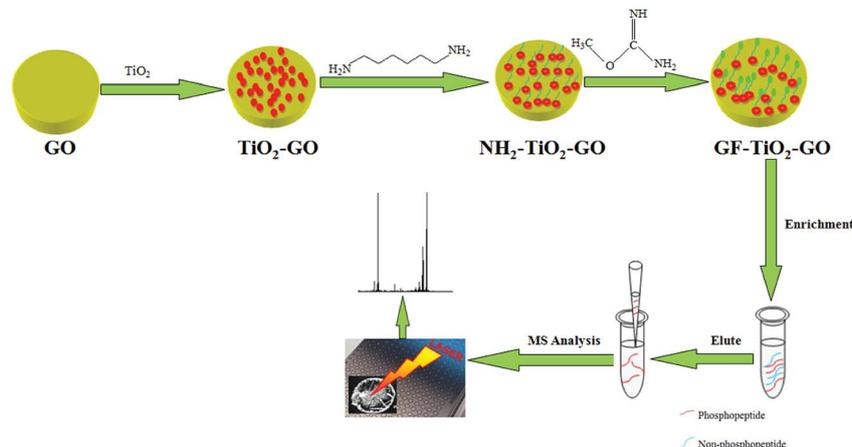
Fig. 1 Schematic illustration for preparation of GF-TiO<sub>2</sub>-GO nanohybrids and the typical protocol for phosphopeptide enrichment.
