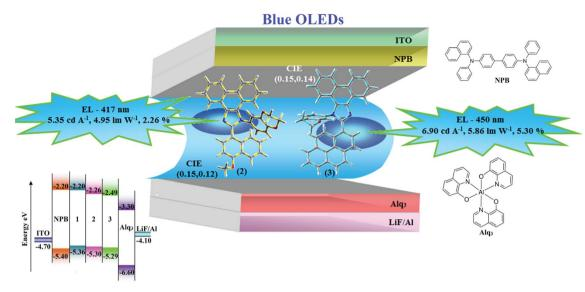
Fig. 6 Energy level and molecular structures of materials used in devices.
