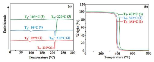
Fig. 3 (a) DSC and (b) TGA graphs of fused polycyclic aryl dihydrobenzodioxin phenanthroimidazoles
