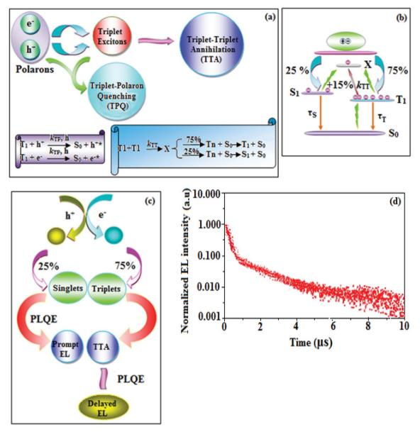
Fig. 9 Schematic representation of (a) triplet-triplet annihilation (TTA)/triplet-polaron guenching (TPQ) processes, (b) spin-statistics in electrically driven OLEDs, (c) delayed emission and (d) transient-EL curve for device III.
