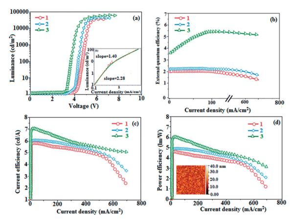
Fig. 7 Device performances: (a) luminance (*L*) versus voltage [inset: roll-off efficiency, device III]; (b) external quantum efficiency ( $\eta_{ex}$ ) versus current density (*J*); (c) current efficiency ( $\eta_{ex}$ ) versus current density (*J*), and (d) power efficiency ( $\eta_{ex}$ ) versus current density (*J*) [inset: AFM image].
