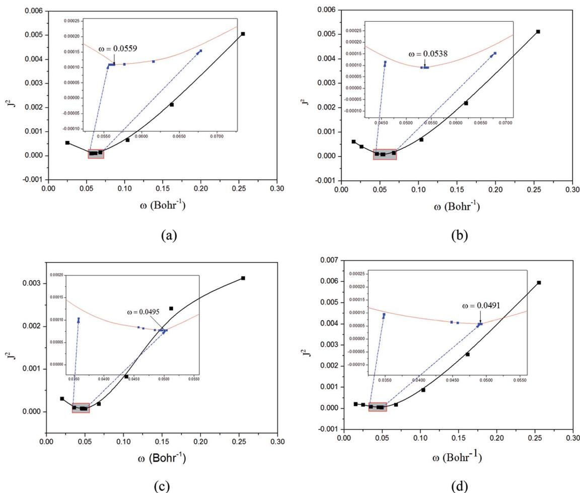
Fig. 3 Functions defined in eqn (2) used for determining of the optimally-tuned range-separation parameter  $\omega$  ( $\text{bohr}^{-1}$ ) at the  $\text{LC-BLYP}_{\alpha=0.0,\beta=1.0}^*/6-31+G(d)$  level in the solid state. (a)  $\text{Cu}(\text{pop})(\text{pz}_2\text{BH}_2)$ ; (b)  $\text{Cu}(\text{pop})(\text{pz}_4\text{B})$ ; (c)  $\text{Cu}(\text{pop})(\text{pz}_2\text{Bph}_2)$ ; (d)  $\text{Cu}(\text{dppb})(\text{pz}_2\text{Bph}_2)$ .
