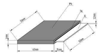
Fig. 1 Schematic illustration of the Pb/Sn/Al laminated composite electrode material.
