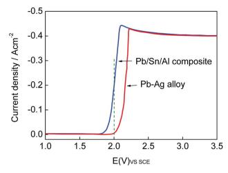
Fig. 7 Linear scanning voltage-current curves of the Pb/Sn/Al composite and Pb-Ag alloy.
