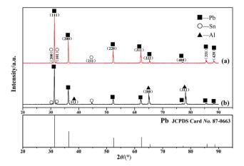
XRD patterns of the interface at the (a) Pb side and (b) Al side.
