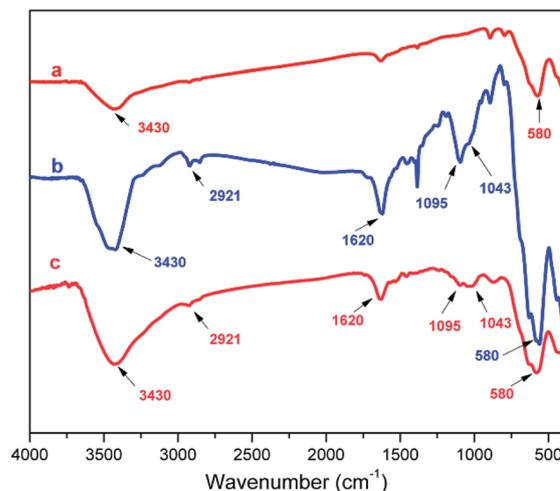
Fig. 1 FT-IR spectra of  $\text{Fe}_3\text{O}_4$  (a), primitively prepared LAIL@MNP (b), and the LAIL@MNP sample after the fifth recovery (c).
