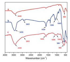
Fig. 1 FT-IR spectra of Fe<sub>3</sub>O<sub>4</sub> (a), primitively prepared LAIL@MNP (b), and the LAIL@MNP sample after the fifth recovery (c).
