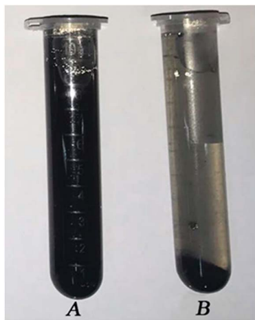
Fig. 8 The photographs of the GNPs dispersion which were allowed to stand for one month: (A) modified GNPs and (B) pure GNPs.
