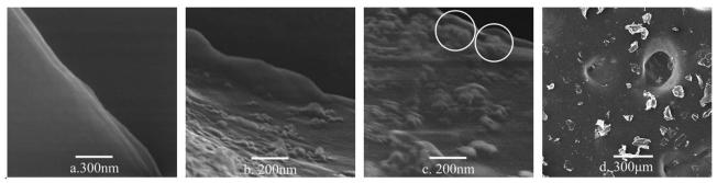
Fig. 4 FESEM micrographs of: (a) pure GNPs, (b) surface of the modified GNPs, (c) edge of the modified GNPs, and (d) the modified GNPs in aqueous solution.
