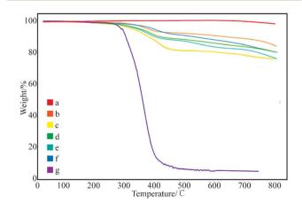
Fig. 5 Thermogravimetric curves of modified GNPs at ultrasonication time: (a) 0 h, (b) 2 h, (c) 4 h, (d) 8 h, (e) 12 h, (f) 24 h, and (g) SMA.
