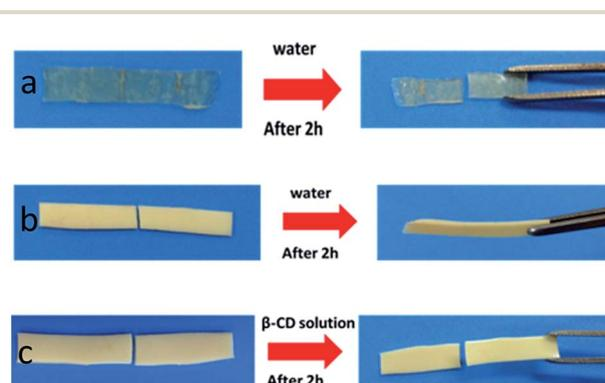
Fig. 10 Self-healing tests using different materials: (a) samples without CD-Al<sub>2</sub>O<sub>3</sub> NPs; (b) samples without PVP; (c) self-healing test of PVP/p(HEMA-co-BA) after smearing cyclodextrin solution at cutting surface.
