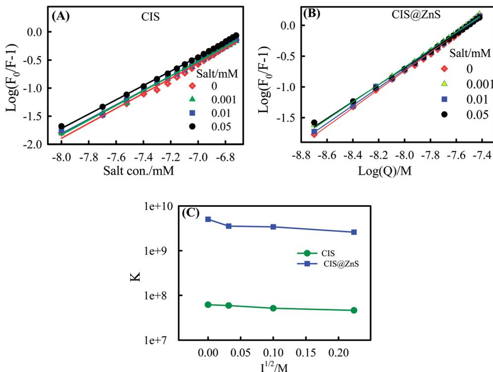
**Fig. 6** (A) Stern–Volmer plot for binding constant obtained from the fluorescence data of lysozyme–CIS complexes as a function of different concentrations of NaCl. (B) Stern–Volmer plot obtained from the fluorescence data of lysozyme–CIS@ZnS complexes as a function of different concentrations of NaCl. (C) Semi-log plot of binding constant of lysozyme–QDs complexes (CIS and CIS@ZnS) as a function of concentration of NaCl.
