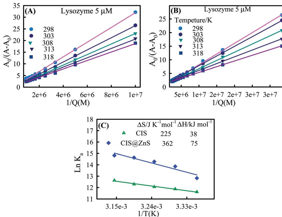
Fig. 5 Double reciprocal (Benesi–Hildebrand) plot for the interaction of lysozyme (5  $\mu\text{M}$ ) and (A) CIS, (B) CIS@ZnS core-shell QDs at different temperatures (298, 303, 308, 313 and 318 K). (C) Semi-log plot (Van't Hoff equation) of rate constant  $K$  against reciprocal temperature for determination of thermodynamic parameters of QD-lysozyme interaction.
