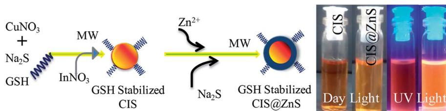
Scheme 1 Schematic representation of the synthesis process of CIS and CIS@ZnS core-shell QDs. Right side photographs of CIS and CIS@ZnS QDs under day and UV light.
