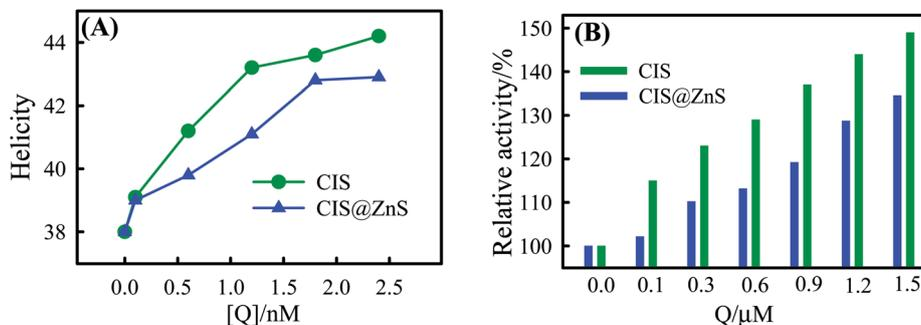
**Fig. 7** Dependence of secondary structure (helicity) of lysozyme (5  $\mu\text{M}$ ) on CIS and CIS@ZnS QD with concentration (0.1 nM to 2.4 nM) at 298 K. Note the gain of secondary structure due to complexation of proteins with QDs. (B) Effect of CIS and CIS@ZnS core–shell QD with concentrations 0.1 to 1.5  $\mu\text{M}$  for CIS and CIS@ZnS QDs, on the enzymatic activity of lysozyme (5  $\mu\text{M}$ ).
