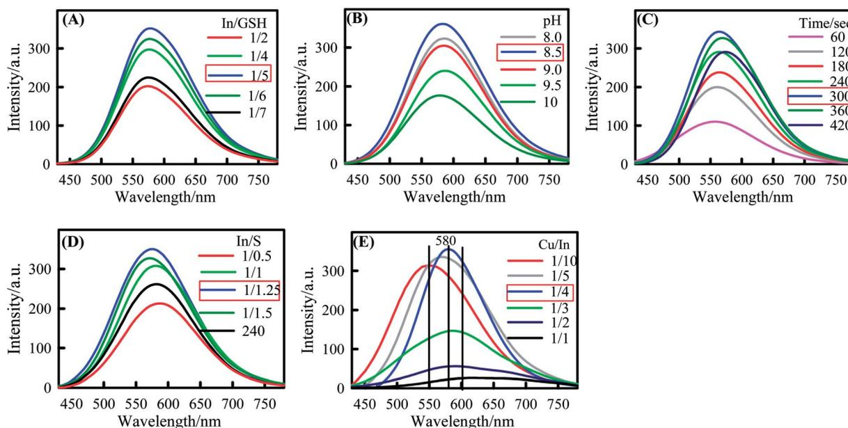
Fig. 1 Fluorescence intensity of the CuInS<sub>2</sub>@ZnS core-shell QDs with different (A) In/GSH ratios, (B) pH value, (C) MW irradiation time, (D) In/S ratios and (E) Cu/In cation ratios. The red-boxed composition refers to the best PLQY value.
