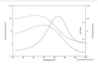
Fig. 4 DMA analysis for Nafion 117 "annealed, H<sub>2</sub>O 100 °C and oriented". Sample parameters: length 13.47 mm, width 5.75 mm, thickness 0.20 mm.
