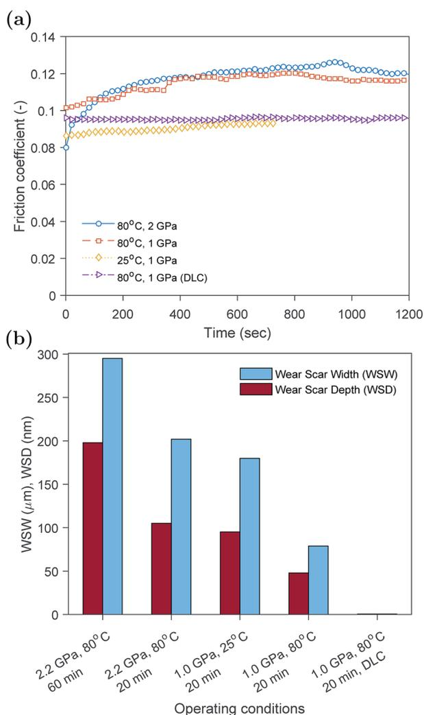
Fig. 2 (a) Evolution of the friction coefficient during the *in situ* tests using plain steel and DLC coated countersurfaces, and (b) wear scar width and depth measured using interferometry technique after removing the tribofilm using EDTA.
