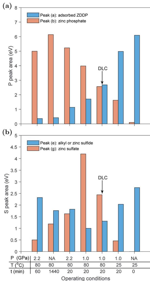
Fig. 8 Comparison between the normalized areas of the main peaks at the (a) P k-edge and (b) S k-edge of the ZDDP tribo- and thermal films at the end of each *in situ* test. All the test were performed using steel–steel countersurfaces except the one indicated by the arrow in which DLC–DLC countersurfaces were used.
