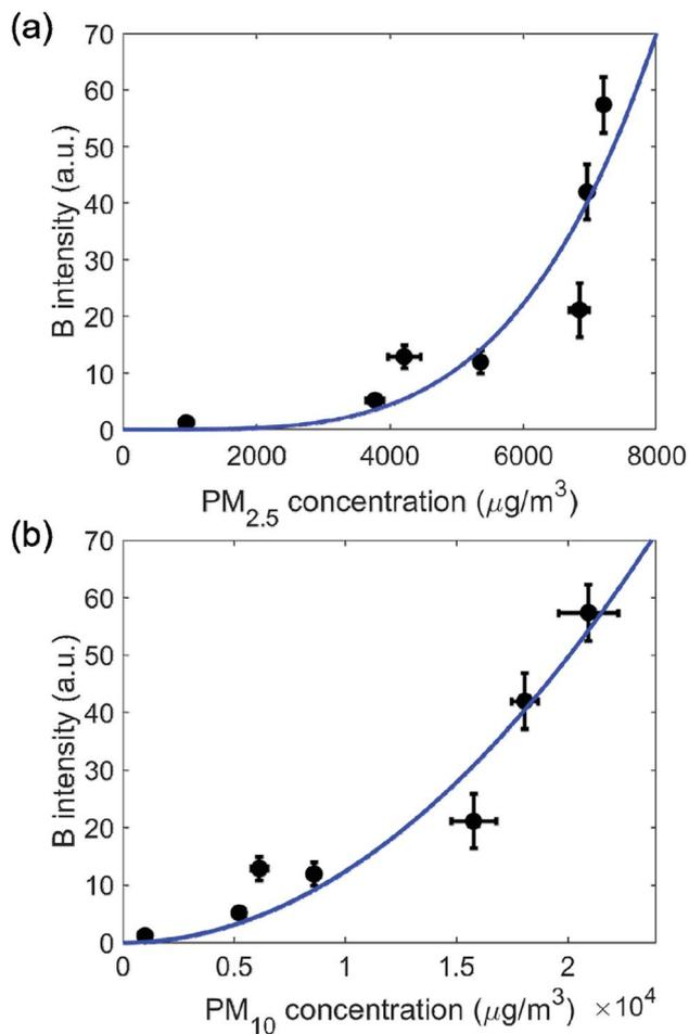
Fig. 2 Calibration line of absolute (a) PM<sub>2.5</sub> and (b) PM<sub>10</sub> concentrations for B component.
