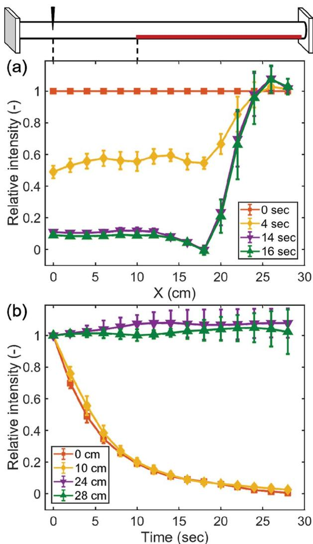
Fig. 4 (a) Spatially resolved PM at the 0<sup>th</sup>, 4<sup>th</sup>, 14<sup>th</sup> and 16<sup>th</sup> second and (b) temporally resolved PM at 0, 10, 24, and 28 cm under stationary mode with a voltage of +13 kV in tubular system with diameter of 3 cm.
