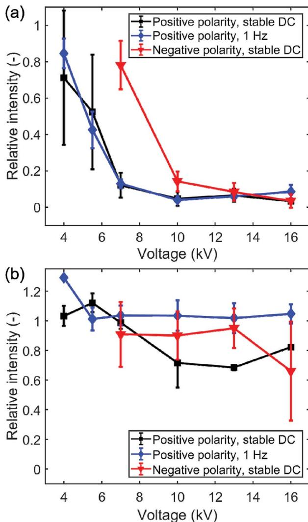
Fig. 5 Relative intensity with different electrical modes and voltage of 4–16 kV at 15<sup>th</sup> second and at (a) 6 cm and (b) 26 cm under stationary mode in tubular system with diameter of 3 cm.
